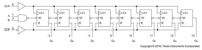
Figure 4. Logic Diagram
