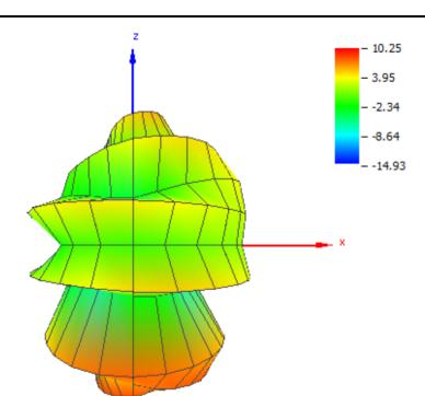
Figure 12. Radiation Pattern Plot Top
