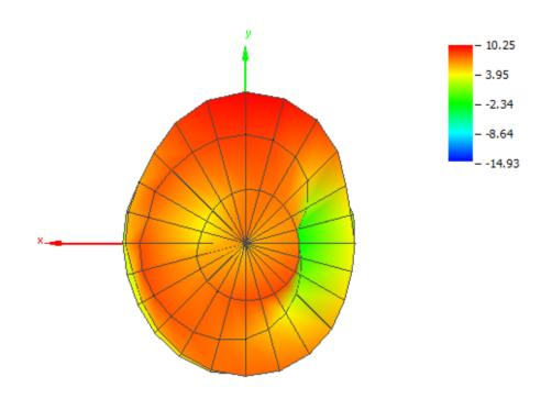
Figure 9. Radiation Plot Pattern Back
