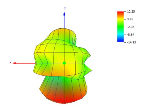
Figure 13. Radiation Pattern Plot Bottom
