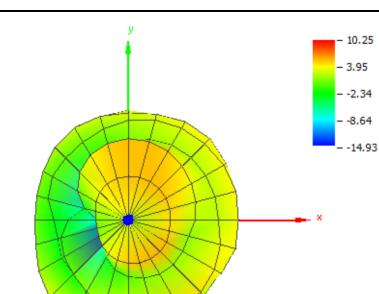
Figure 8. Radiation Pattern Plot Front
