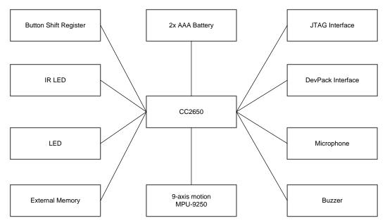
Figure 1. CC2650 Remote Control Block Diagram
