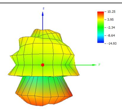
Figure 10. Radiation Pattern Plot Right Side
