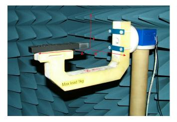
Figure 6. DUT Mounted on Rotating Arm
