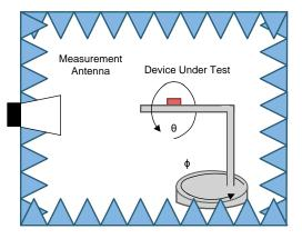
Figure 5. Antenna Radiation Pattern
