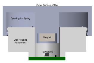
Figure 2-6. Magnetic Dial Push Button Stackup
