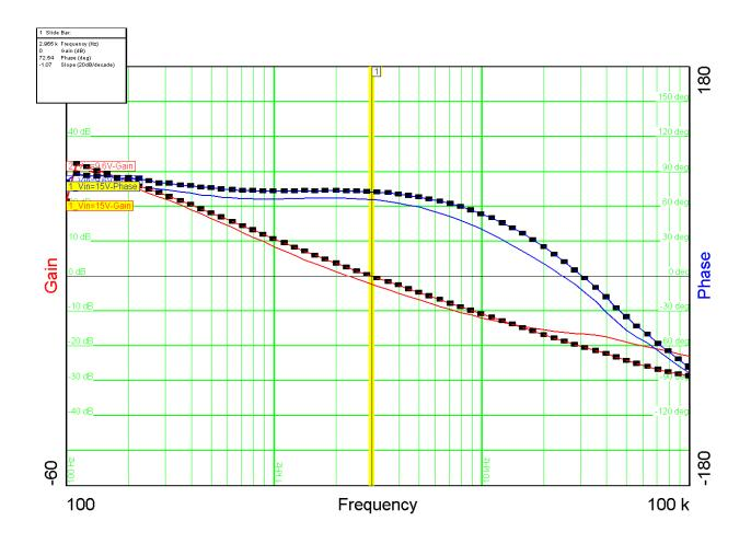
Input voltage = 15V Phase margin = 72.5deg Bandwidth = 2.97kHz
