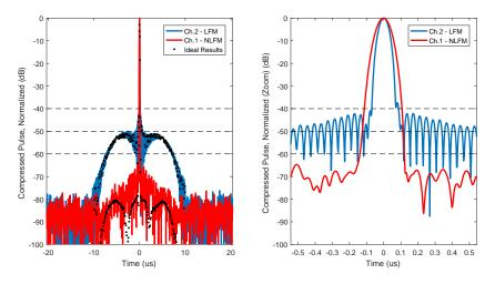
Figure 13. Measured Output of Pulse-Compression Filters
