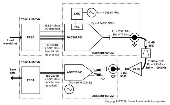
Figure 8. Measurement Test Setup
