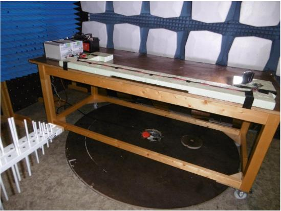
Figure 26. CISPR 25 Radiated Emissions Setup
