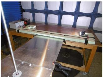
Figure 24. CISPR 25 Conducted Emissions Setup
