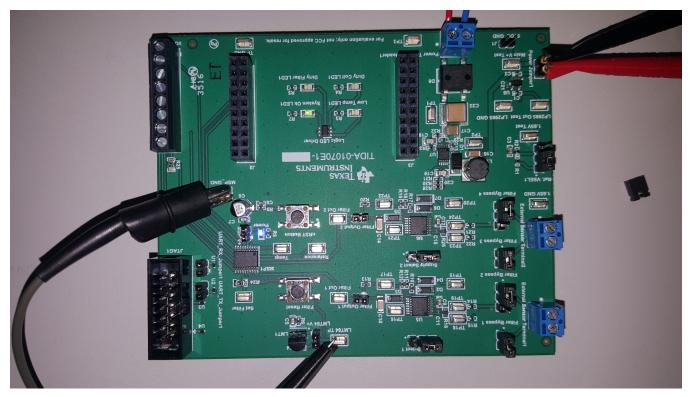
Figure 37. TIDA-01070 Current Consumption Test Setup
