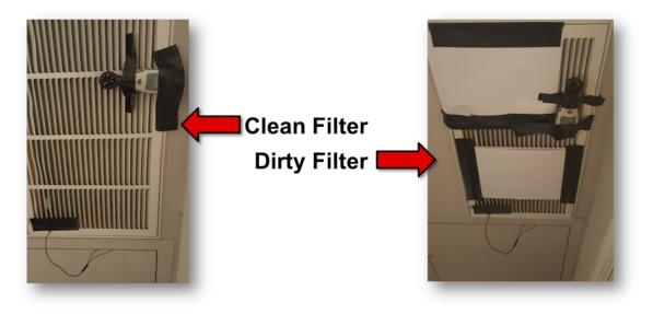
Figure 26. Filter Condition Test Setup
