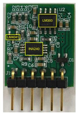
Figure 7. Top View of TIDA-01141
