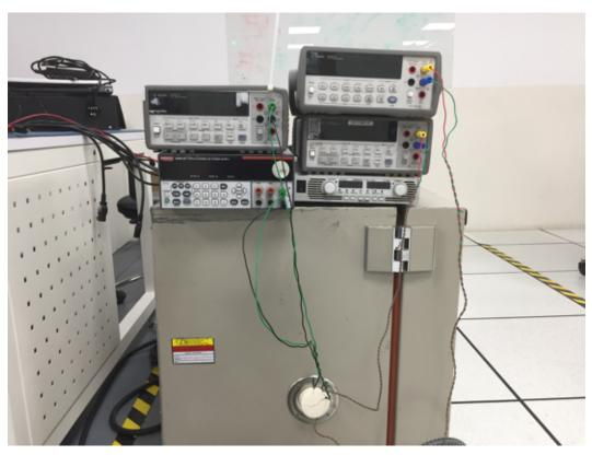
Figure 9. Test Setup for Testing Across Temperature Range
