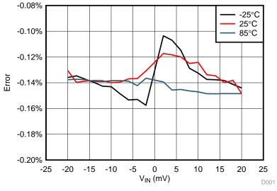
Figure 11. Accuracy of Current Sensing System
