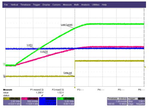
Figure 17. Comparator Output for Output Voltage Crossing V-HTV
