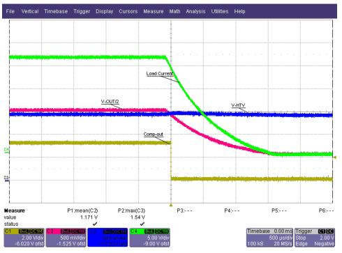
Figure 18. Comparator Output for Output Voltage Below V-HTV
