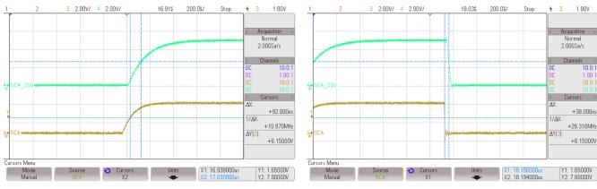
Figure 42. Rising Edge Propagation Delay of ISO1541
