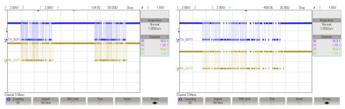
Figure 28. CAN Multiple Data Packet Communication
