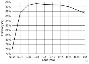
Figure 49. Efficiency of Auxiliary Power Supply
