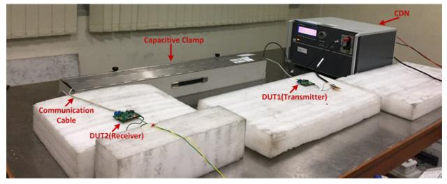
Figure 44. EFT Test Setup
