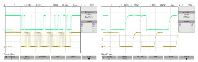
Figure 38. I2C Output Clock and Data
