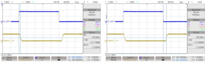
Figure 34. Rising Edge Propagation Delay of ISO1050
