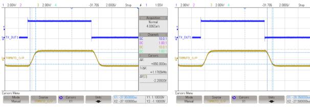
Figure 26. Rise Time of Terminated Output of ISO3082
