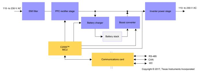
A typical block diagram of an online UPS (double conversion UPS) is shown in Figure 1:
