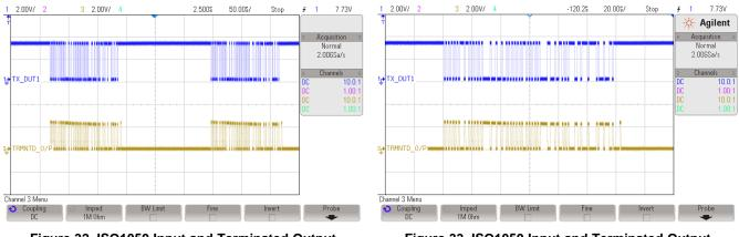
Figure 32. ISO1050 Input and Terminated Output Waveform (Multiple Data Packets)
