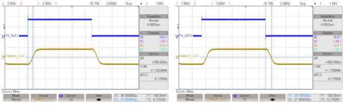
Figure 24. Rising Edge Propagation Delay of ISO3082
