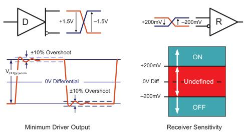
Figure 3. RS-485 Specified Bus Signal Levels
