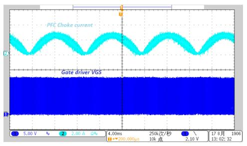
Figure 20. Choke Current and VGS Waveform at Line Frequency Scale
