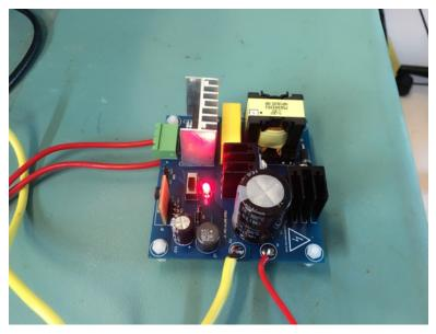
Figure 3. Operating AC/DC Converter on Test Bench
