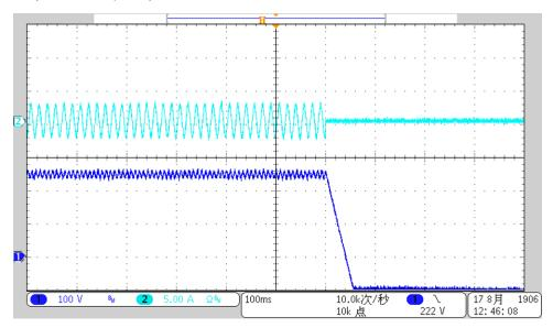
Figure 14. Shutdown Behavior for 230-V AC 60-Hz Input Voltage
