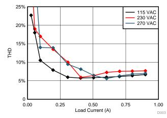
Figure 6. THDi versus Load Current
