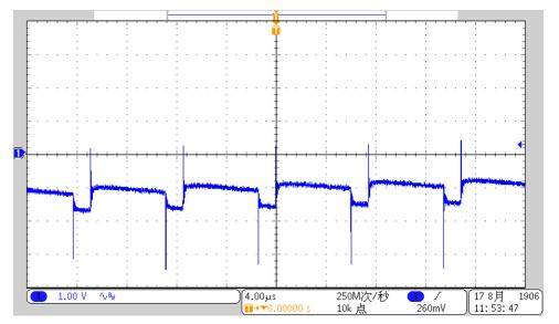
Figure 19. Output Voltage Ripple at Switching Frequency for 60-Hz Line Frequency
