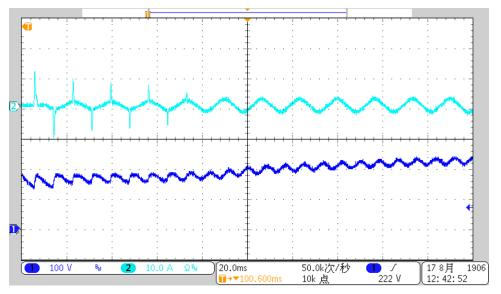
Figure 13. Startup Behavior for 230-V AC 60-Hz Input Voltage
