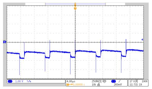
Figure 18. Output Voltage Ripple at Switching Frequency for 50-Hz Line Frequency
