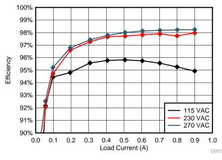
Figure 4. Efficiency versus Load Current
