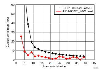
Figure 8. Current Harmonic Limit and Converter Current for 10% Rated Output Power
