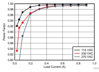
Figure 5. Power Factor versus Load Current
