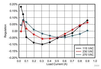
Figure 7. Relative Output Voltage Regulation versus Load Current
