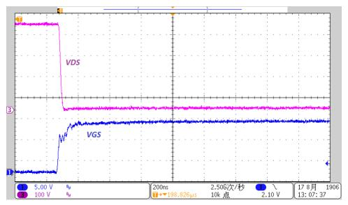
Figure 22. VGS and VDS MOSFET Turnon Waveforms
