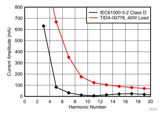
Figure 10. Current Harmonic Under 350-W Input
