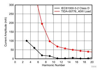
Figure 9. Current Harmonic for 200-W Input Power
