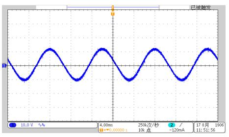
Figure 16. 50-Hz Line Frequency Output Voltage Ripple
