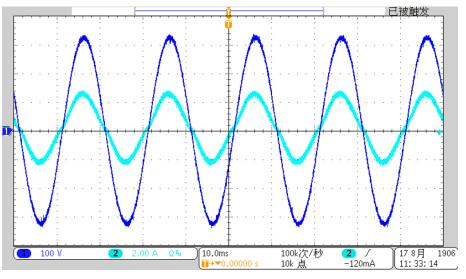
Figure 15. Input Voltage and Current for Full Load With 230-V AC Input
