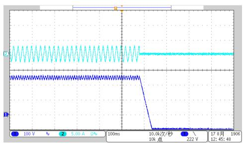
Figure 12. Shutdown Behavior for 230-V AC 50-Hz Input Voltage
