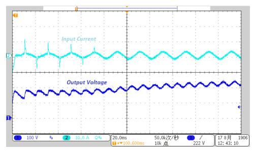
Figure 11. Startup Behavior for 230-V AC 50-Hz Line Voltage Input
