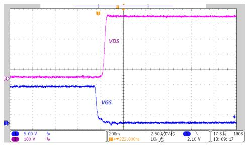
Figure 23. VGS and VDS MOSFET Turnoff Waveforms
