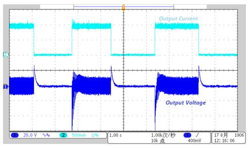
Figure 24. Load Transient Under 230-V Input
