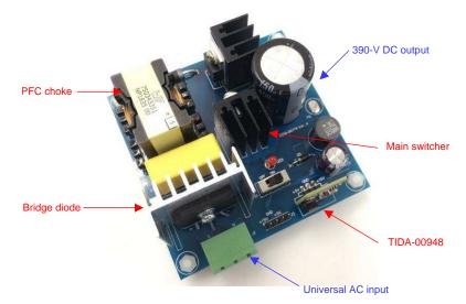
Figure 2. TIDA-00776 PCB With Functional Blocks
