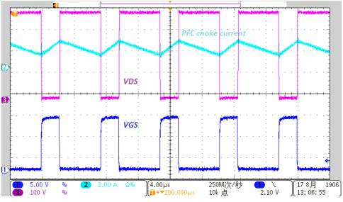
Figure 21. Choke Current, VGS, and VDS at Switching Frequency Scale
