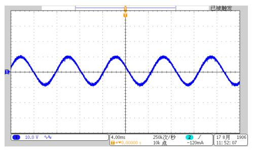
Figure 17. 60-Hz Line Frequency Output Voltage Ripple
