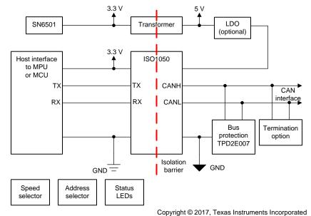
Figure 2. CANopen Block Diagram
