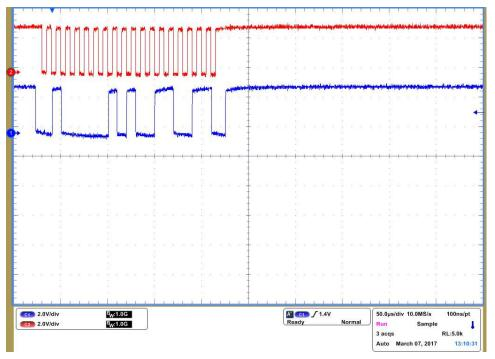
Figure 13. I<sup>2</sup>C Communication
