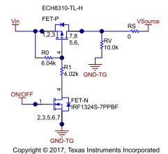
Figure 13. Socket Board ON and OFF Logic
