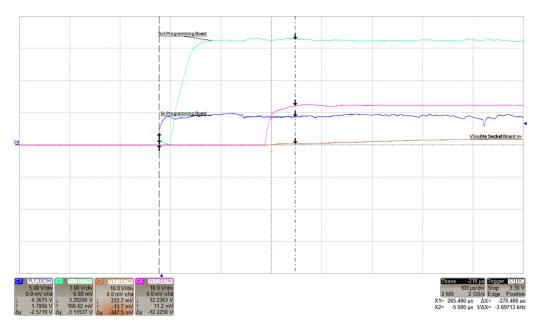
Figure 17. VSource Socket Board Start-up Time: 270 µs
