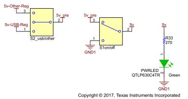
Figure 4. TIDA-01373 System Control Switches—Programming Board
