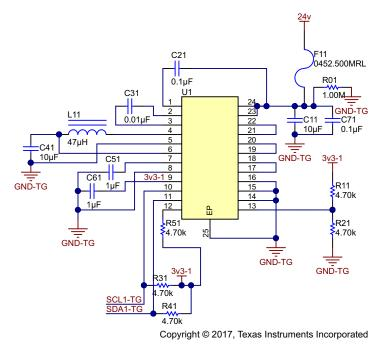
Figure 14. DRV10983-Q1 Socket Schematic
