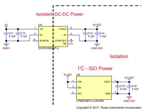
Figure 10. Power Isolation Circuitry—Programming Board
