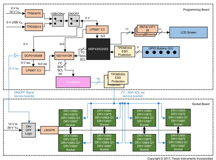
Figure 1. TIDA-01373 Block Diagram
