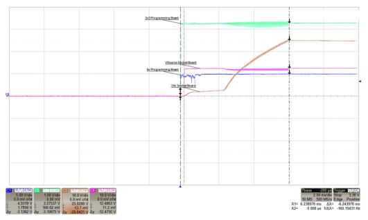
Figure 18. 24-V Socket Board Startup Time: 6.24 ms
