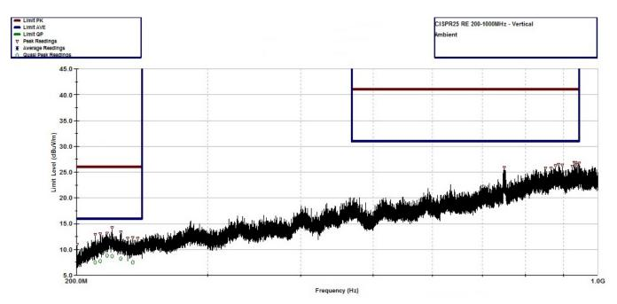
Figure 39. CISPR 25 Radiated Emissions: 200 MHz to 1 GHz, Vertical Antenna Orientation, Ambient Scan
