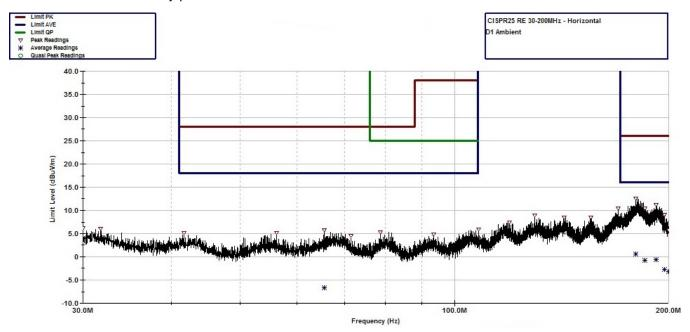
Figure 34. CISPR 25 Radiated Emissions: 30 MHz to 200 MHz, Horizontal Antenna Orientation, Ambient Scan
