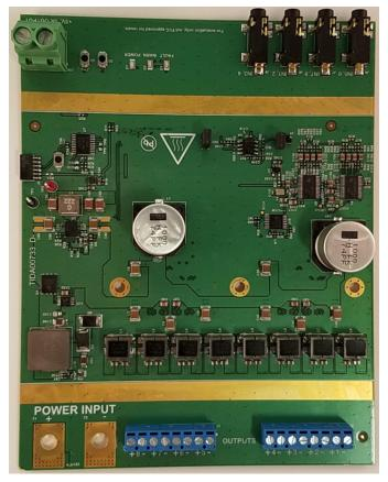
Figure 24. Connectors for TIDA-00733 Assembly
