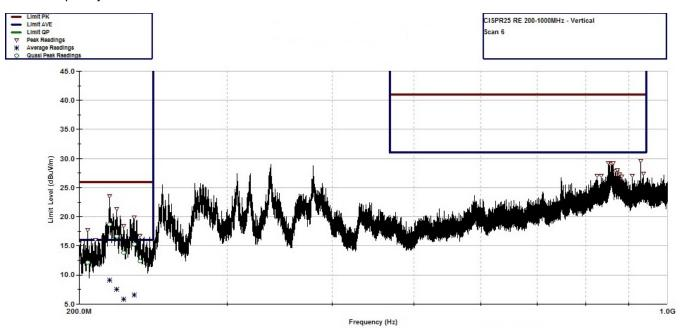
Figure 41. CISPR 25 Radiated Emissions: 200 MHz to 1 GHz, Vertical Antenna Orientation
