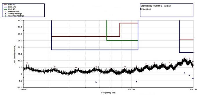
Figure 35. CISPR 25 Radiated Emissions: 30 MHz to 200 MHz, Vertical Antenna Orientation, Ambient Scan
