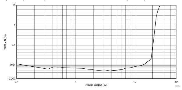
Figure 31. Power Output (W) versus THD + Noise (%) into 4  $\Omega$
