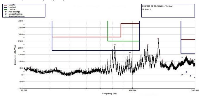
Figure 37. CISPR 25 Radiated Emissions: 30 MHz to 200 MHz, Vertical Antenna Orientation
