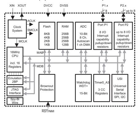
Figure 10. MSP430G2332 Functional Block Diagram
