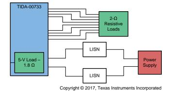
Figure 28. Test Setup Block Diagram for EMI Tests
