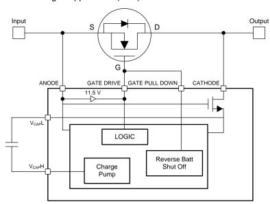
Figure 7. LM74610-Q1 Functional Block Diagram
