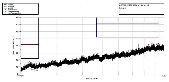
Figure 38. CISPR 25 Radiated Emissions: 200 MHz to 1 GHz, Horizontal Antenna Orientation, Ambient Scan
