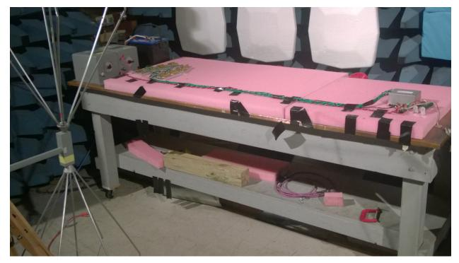
Figure 29. Radiated Emissions Test Setup
