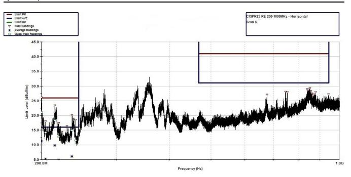
Figure 40. CISPR 25 Radiated Emissions: 200 MHz to 1 GHz, Horizontal Antenna Orientation
