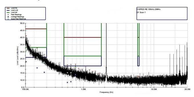
Figure 33. CISPR 25 Radiated Emissions: 150 kHz to 30 MHz
