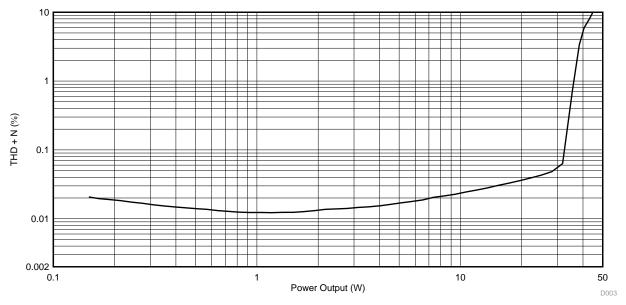
Figure 30. Power Output (W) vs THD + Noise (%) into 2  $\Omega$
