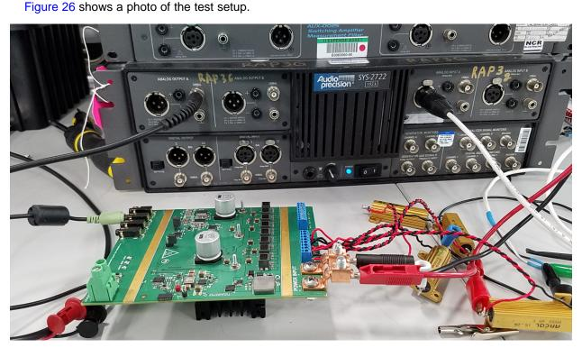
Figure 26. Test Setup for Power Output and Total Harmonic Distortion and Noise Tests
