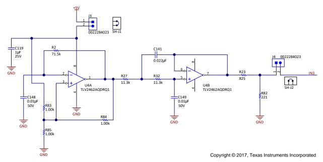
Figure 21. TLV2462-Q1 Oscillator Circuit
