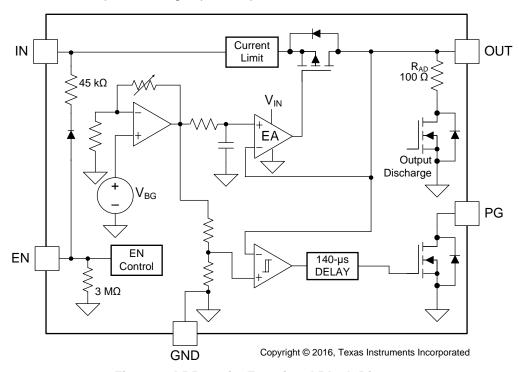
Figure 6. LP5912-Q1 Functional Block Diagram
