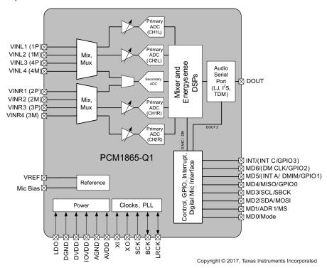
Figure 4. PCM1865-Q1 Simplified Block Diagram
