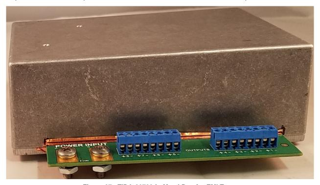
Figure 27. TIDA-00733 in Metal Box for EMI Tests
