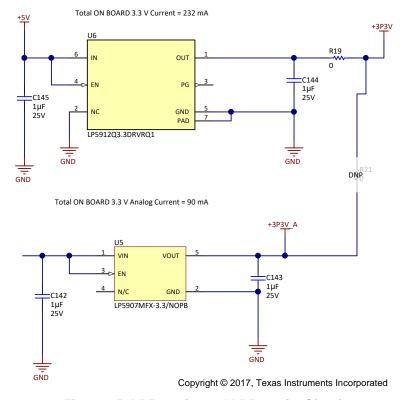
Figure 15. LP5912-Q1 and LP5907-Q1 Circuits
