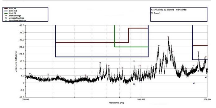
Figure 36. CISPR 25 Radiated Emissions: 30 MHz to 200 MHz, Horizontal Antenna Orientation
