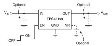
Figure 4. TPS73118 Typical Application Circuit
