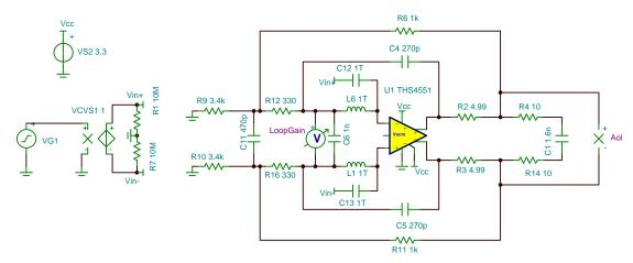
Figure 10. THS4551 TINA-TI Stability Schematic
