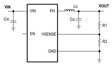
Figure 3. TPS560200 Simplified Schematic
