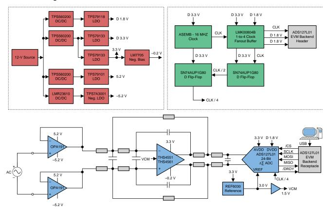
Figure 1. TIDA-01013 Block Diagram
