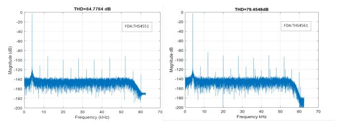
Figure 30. TIDA-01013 Fast-Fourier Transform for 10-V<sub>P</sub>, 4-kHz Sine Wave Input
