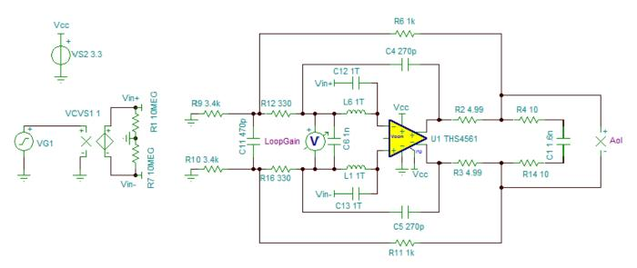
Figure 12. THS4561 TINA-TI Stability Schematic
