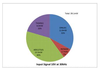
Figure 32. TIDA-01013 AFE (THS4561) and ADC Power Consumption
