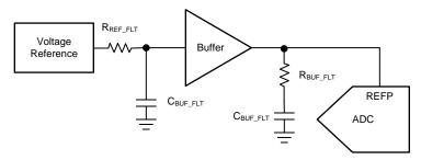
Figure 14. Simplified Schematic of Reference Driver
