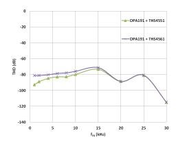
Figure 28. TIDA-01013 THD Versus Input Signal Frequency
