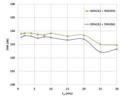
Figure 27. TIDA-01013 SNR Versus Input Signal Frequency
