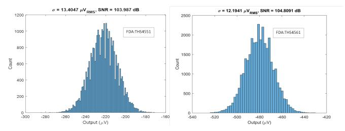
Figure 29. TIDA-01013 Noise Histogram for 0-V DC Input
