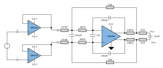
Figure 21. TIDA-01013 AFE Power Simulation Schematic
