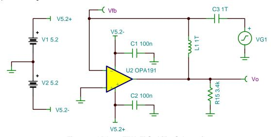
Figure 7. OPA191 TINA-TI Stability Schematic
