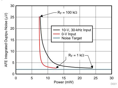
Figure 22. TIDA-01013 AFE Integrated Output Noise versus Power Plot
