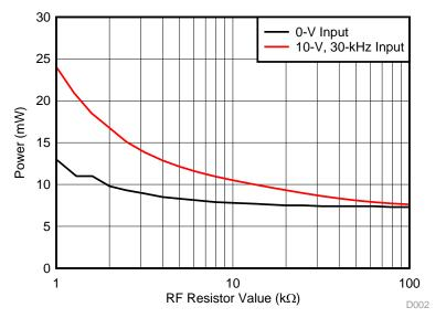
Figure 23. TIDA-01013 AFE Power versus R<sub>F</sub> Resistance
