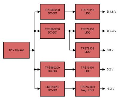
Figure 16. TIDA-01013 Power Supply Block Diagram
