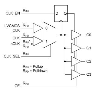
Figure 5. LMK00804 Simplified Schematic
