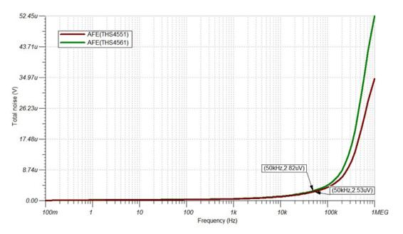
Figure 20. TIDA-01013 AFE Output Noise
