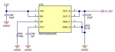
Figure 15. Reference Voltage Altium Schematic
