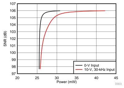
Figure 24. TIDA-01013 System SNR versus Power Plot
