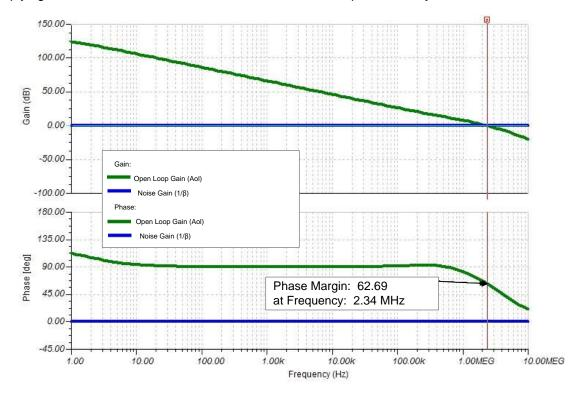
Figure 8. OPA191 TINA-TI Stability Simulation Results
