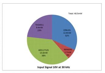
Figure 31. TIDA-01013 AFE (THS4551) and ADC Power Consumption
