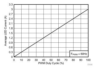
Figure 15. LED Current versus PWM Duty Cycle (0% to 100%)
