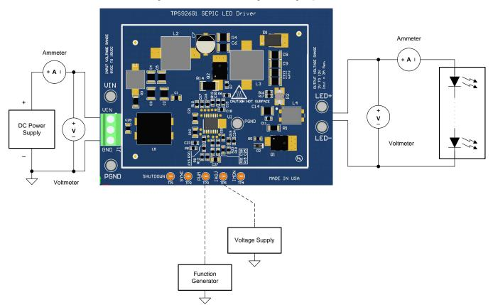
Figure 5. Test Setup Connections
