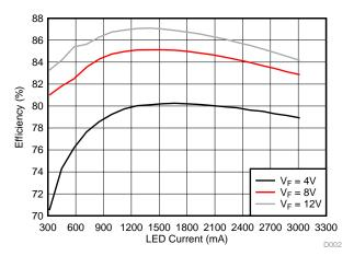
Figure 11. 13-V Input Efficiency versus LED Current
