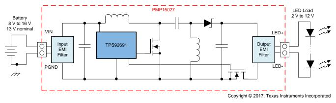
Figure 1. PMP15027 Block Diagram
