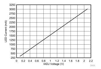
Figure 14. LED Current versus IADJ Voltage (IADJ Varied From 0.1 V to 2.1 V)
