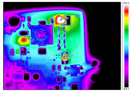
Figure 16. Thermal Scan—Top-View (Power Components): V<sub>IN</sub> = 13 V, Six LEDs, I<sub>LED</sub> = 3 A
