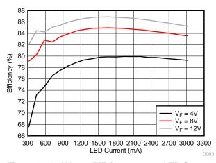
Figure 12. 16-V Input Efficiency versus LED Current
