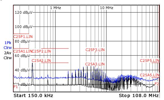
Figure 4. CISPR-25 Class 3 Conducted EMI Scan (C25Px: Peak Limits, C25Ax: Average Limits)  $V_{IN} = 13 V$ ,  $V_F = 12 V$ ,  $I_{LED} = 3 A$  (Pre-Compliance Data)
