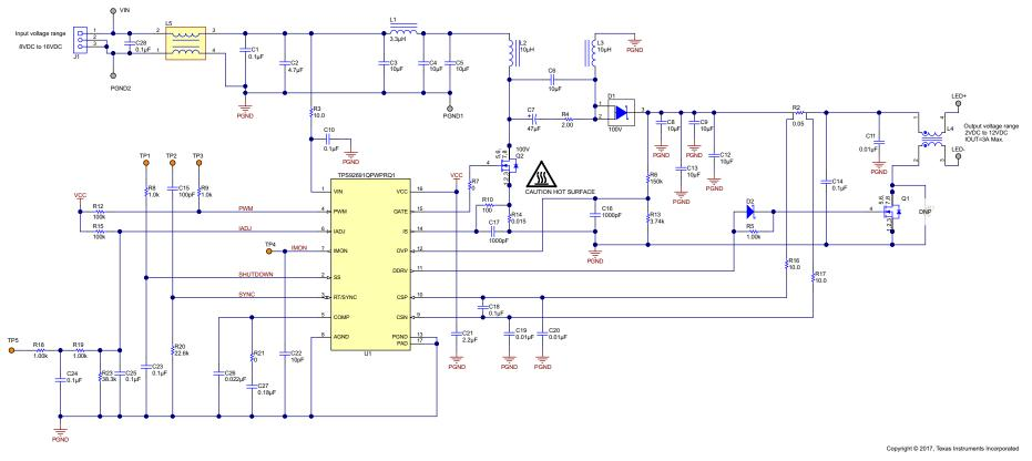
Figure 3. PMP15027 Schematic (R1 Not Populated for PWM Dimming)
