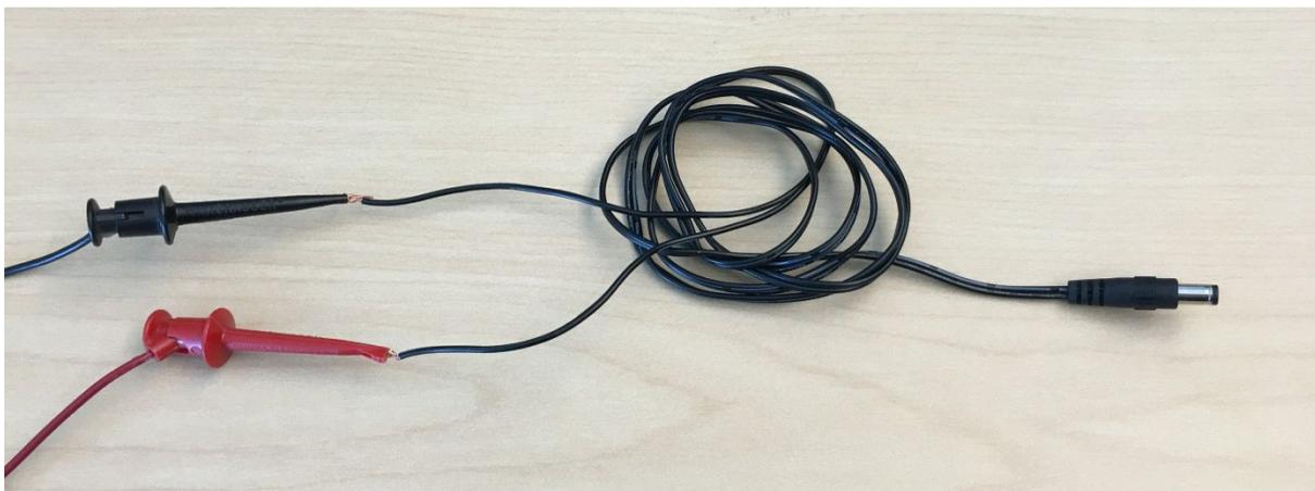
**Figure 22. Power Cable Connection to Bench Meter**
