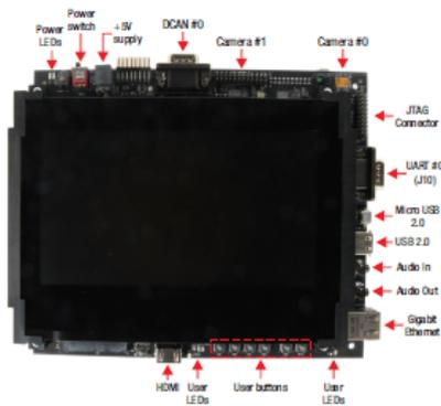
Figure 7. AM437x GP EVM Top View
