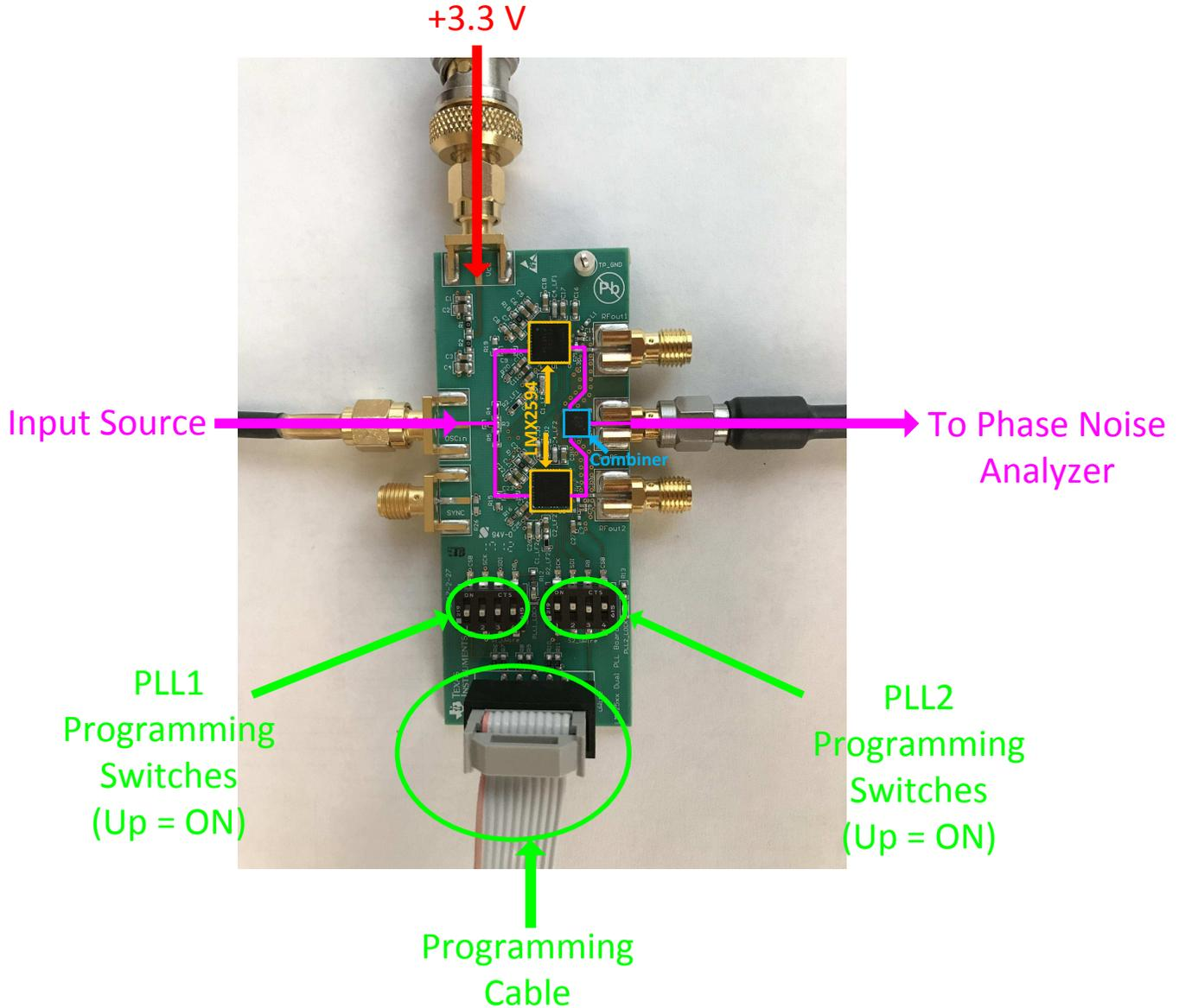
Figure 3. Hardware Setup
