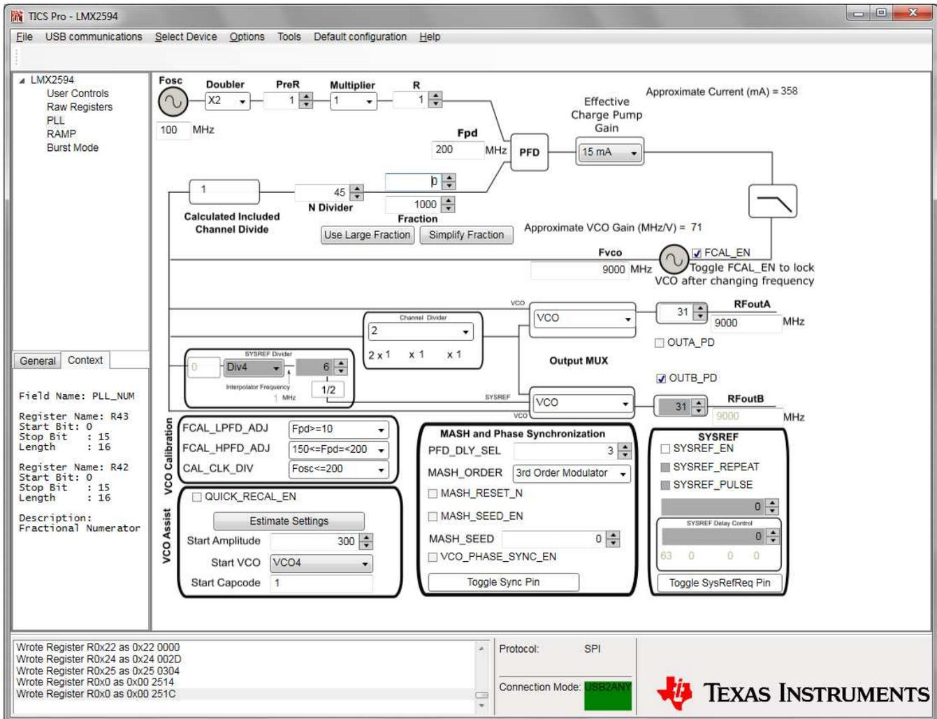
The screenshot displays the TICS Pro software interface for the LMX2594 device. The main window shows a block diagram of the PLL configuration. Key parameters include:
