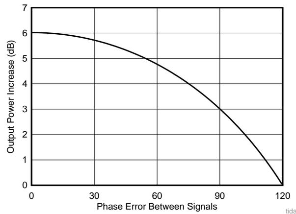
Figure 2. Theoretical Power Increase by Combining Two Signals
