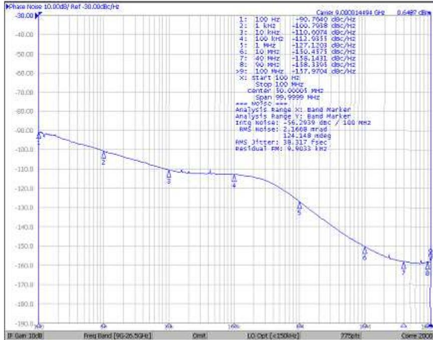
Figure 6. Combination Board Results at 9 GHz
