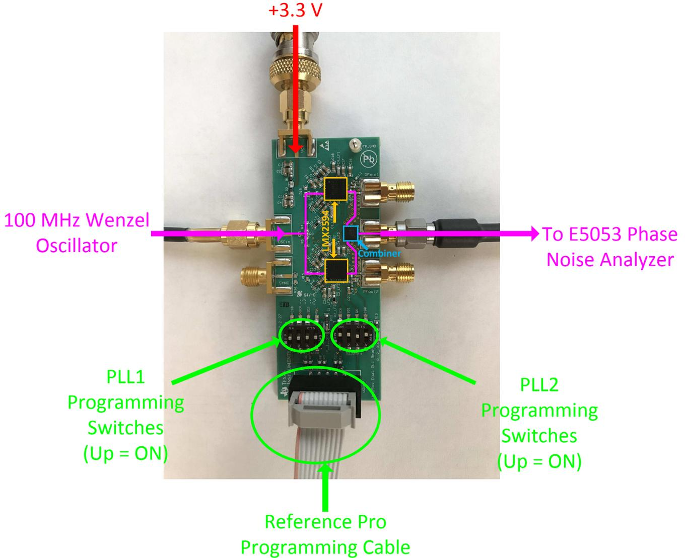
Figure 5. Test Setup
