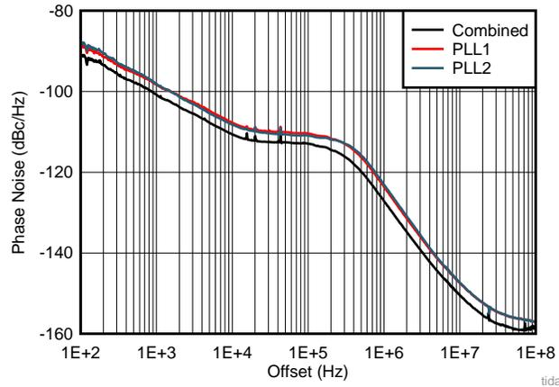
Figure 7. Phase Noise of Combined and Individual PLLs
