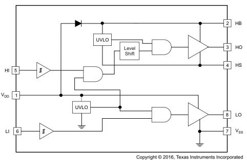
Figure 5. UCC27211D Functional Block Diagram
