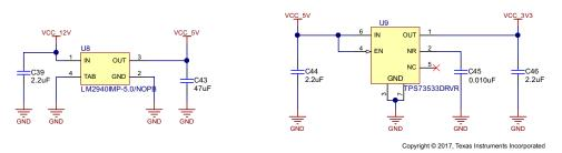
Figure 8. 5-V and 3.3-V Power Supply Schematic
