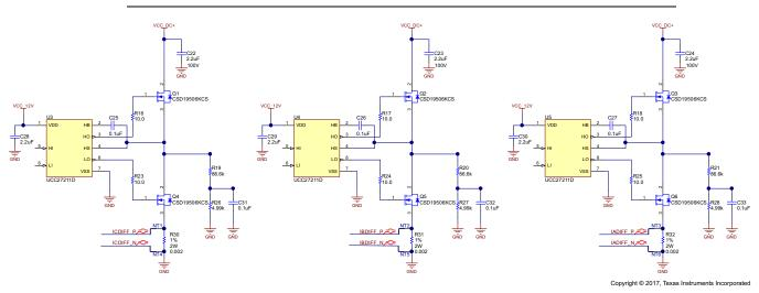
Figure 9. Three-Phase Inverter and MOSFET Gate Driver Schematic
