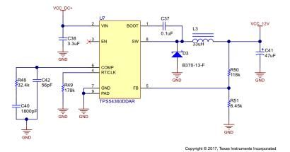
Figure 7. 12-V Power Supply Schematic
