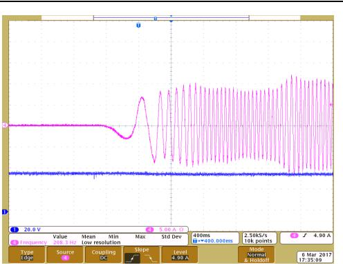
Figure 20. Motor Startup With Light Load
