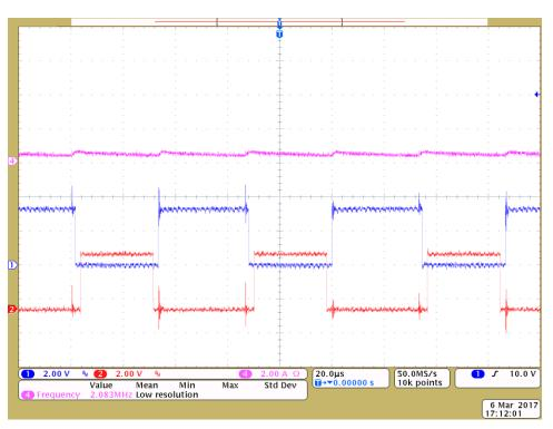
Figure 15. High-Side and Low-Side Gate With Dead Band From MCU
