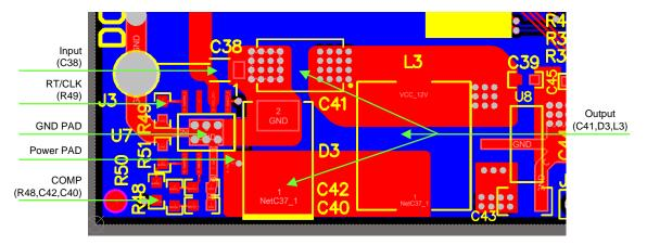
Figure 22. TPS54360 PCB Layout Recommendations
