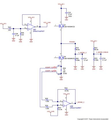
Figure 10. Phase Current and Voltage Sampling Circuit Schematic
