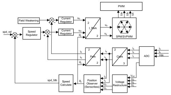
Figure 1. Block Diagram of FOC
