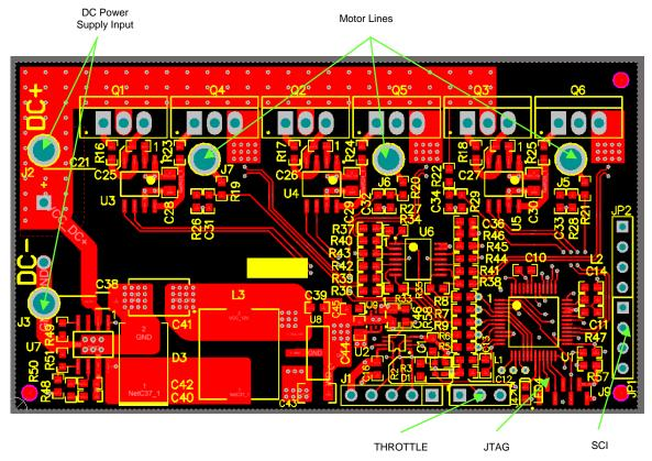
Figure 11. Drive Controller Connections
