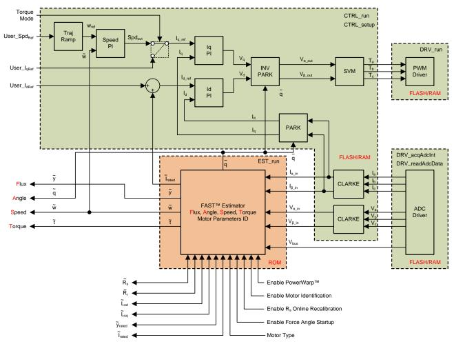
Figure 2. Block Diagram of InstaSPIN-FOC
