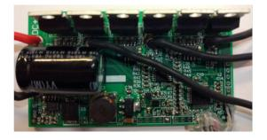
Low-Voltage, 50-A Sensorless FOC for Brushless DC or Permanent-Magnet Synchronous Motors Reference Design Copyright © 2017, Texas Instruments Incorporated 1
