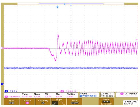
Figure 19. Motor Startup Without Load
