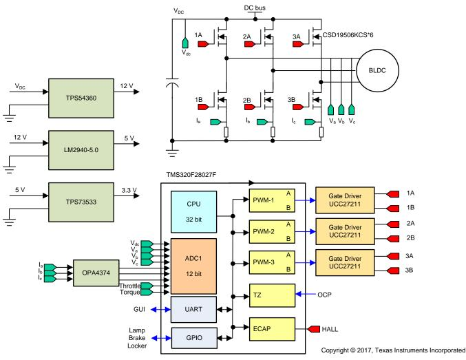
Figure 3. Drive Controller Block Diagram
