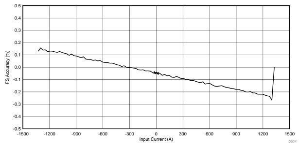
Figure 41. Full-Scale Accuracy in % at 50°C for -1500 A to +1500 A at 14.4 kSPS
