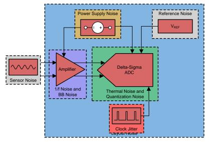
Figure 20. Current Sensor System Noise Sources
