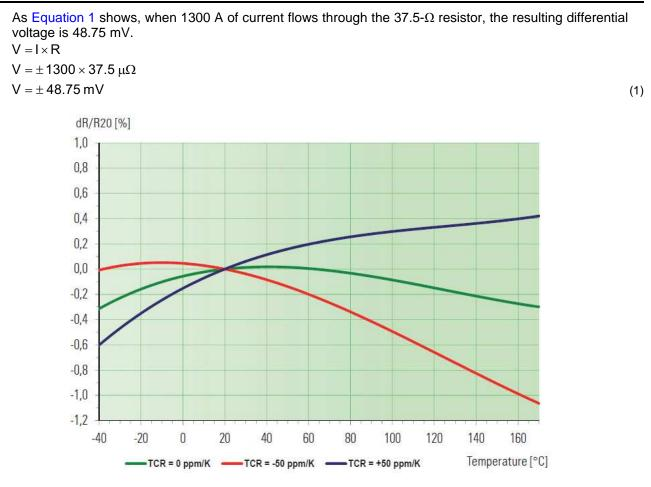
Figure 8. Resistance Change With Respect to Temperation Variations
