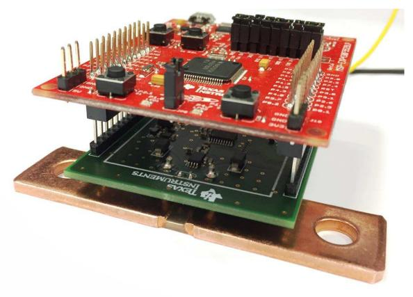
Figure 26. TIDA-03050 Board With MSP430F5529 LaunchPad™
