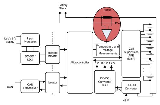
Figure 3. Current Sensor Location in Battery Control Unit
