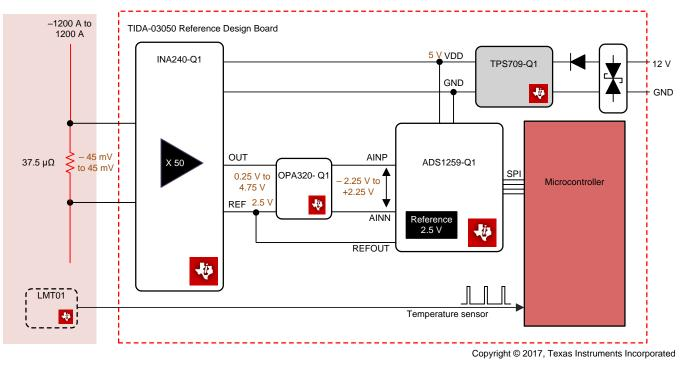
Figure 1. TIDA-03050 Block Diagram
