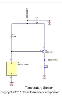
Figure 19. Temperature Sensor Schematic
