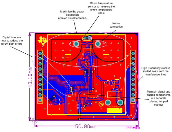
Figure 24. PCB Layout Guidelines
