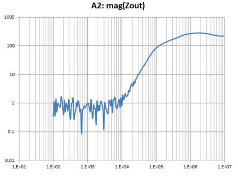
Figure 13. Output Impedance From INA240 Device (Real)
