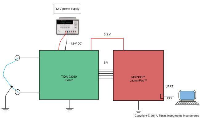
Figure 28. Input Terminals Shorted to Ground
