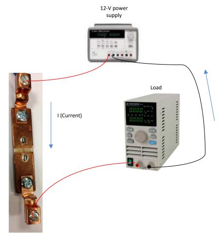
Figure 27. Shunt Value Measurement
