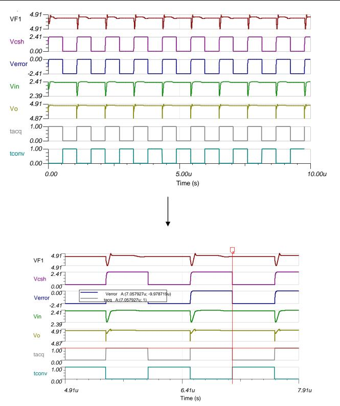
Figure 17. Voltage Signal Levels When INA240 Output is Connected to ADS1259 Through OPA320-Q1
