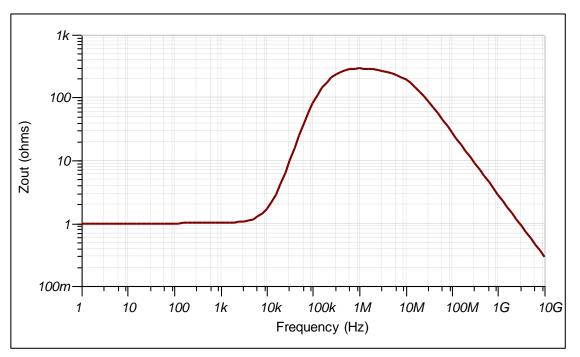
Figure 12. INA240 Output Impedance Block Realization in INA240
