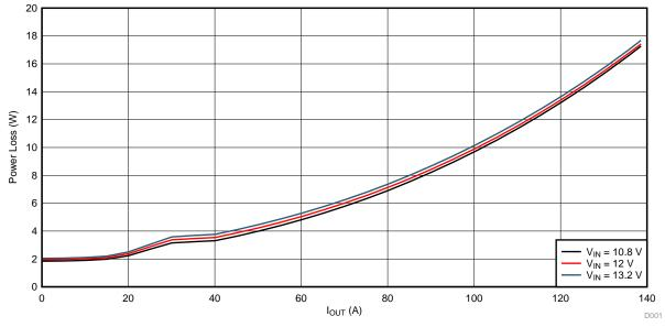
Figure 4. PMP20176 Power Loss Curves:  $V_{out}$  = 0.9 V, 400 kHz
