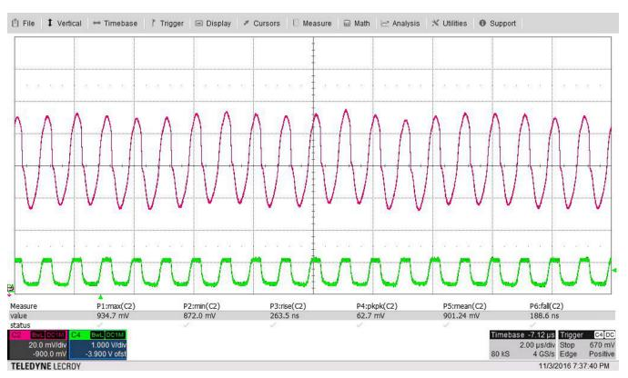
Figure 11. 4-A to 79-A Transient, 1-MHz Load Frequency
