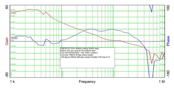
Figure 7. Bode Plot: 50-A Load,  $V_{IN}$  = 12 V
