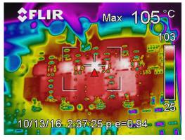
Figure 8. 100-A Load Thermal Performance, No Airflow
