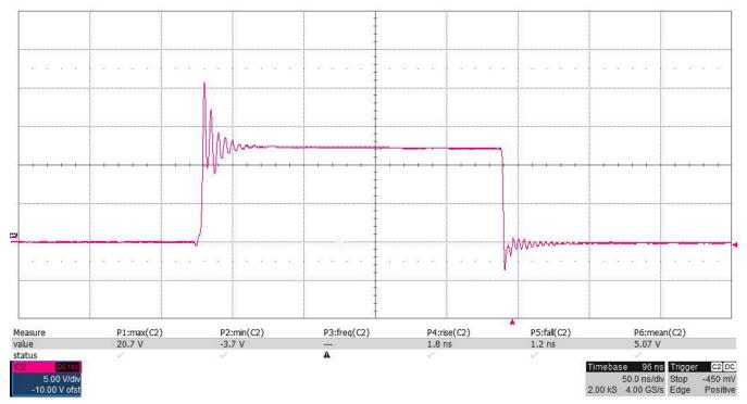
Figure 5. Phase Node Ringing With 40-A Load
