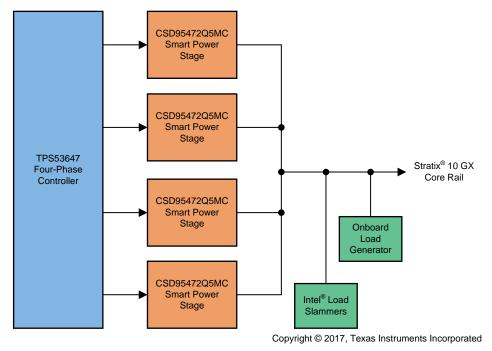
Figure 1. PMP20176 Block Diagram
