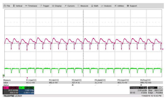
Figure 13. 65-A to 140-A Transient, 1-MHz Load Frequency
