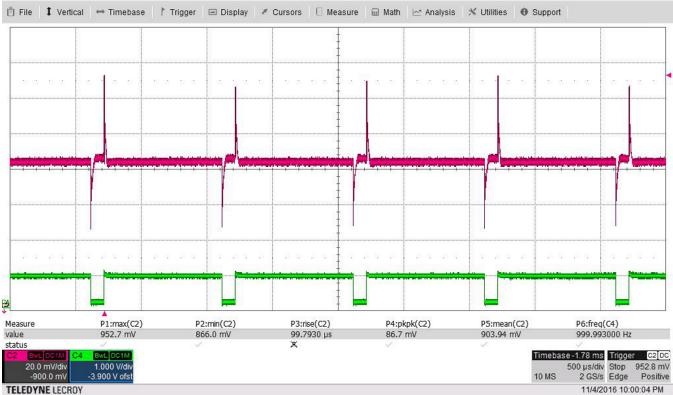
Figure 12. 65-A to 140-A Transient, 1-kHz Load Frequency
