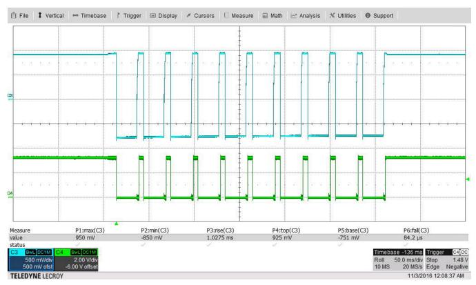
Figure 19. Overcurrent Shutdown With Hiccup Mode
