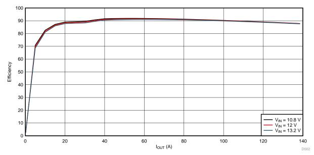
Figure 3. PMP20176 Efficiency Curves: V<sub>OUT</sub> = 0.9 V, 400 kHz
