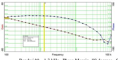
Bandwidth= 1.3 kHz Phase Margin=80 degrees Gain Margin=29dB
