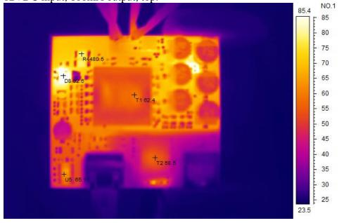
12VDC input, 600mA output, bottom:
