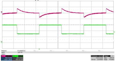
Output load step response, 60mA to 600mA load step, 24VAC input 500mV/div, 200mA/div, 10msec/div, slew rate = 60mA/usec Measured 1.42Vpp across C22:
