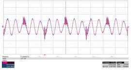
Output ripple, 24VAC input 20mV/div, 5msec/div Measured 66.7mVpp across C22:
