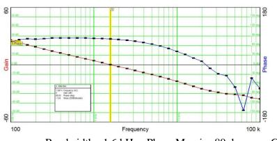
Bandwidth= 1.6 kHz Phase Margin=80 degrees Gain Margin=27dB
