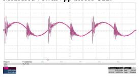
Output ripple, 24VAC input 20mV/div, 5usec/div Measured 46mVpp across C22:
