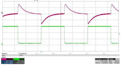
Output load step response, 300mA to 600mA load step, 12VDC input 500mV/div, 200mA/div, 5msec/div, slew rate = 60mA/usec Measured 750mVpp across C22:
