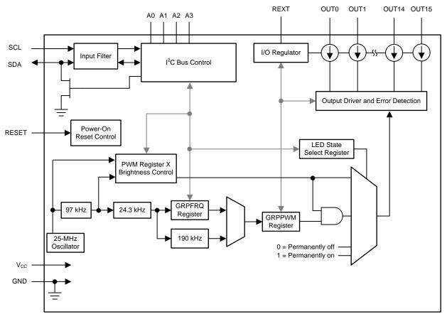
Figure 3. TLC59116-Q1 Block Diagram—OUT0 to OUT15 as Constant Current Sink Outputs
