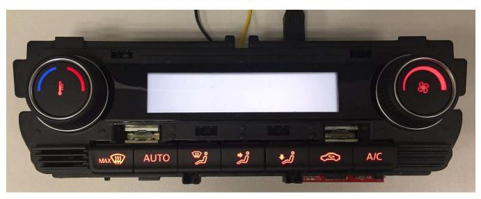
Figure 13. TIDA-01500 into HMI Housing
