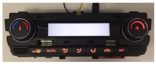
Figure 21. LED Dimming With 80% Duty Cycle
