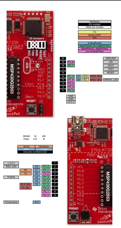
Figure 15. MSP-EXP430G2553 Pinout
