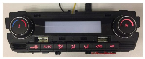
Figure 19. LED Dimming With 20% Duty Cycle
