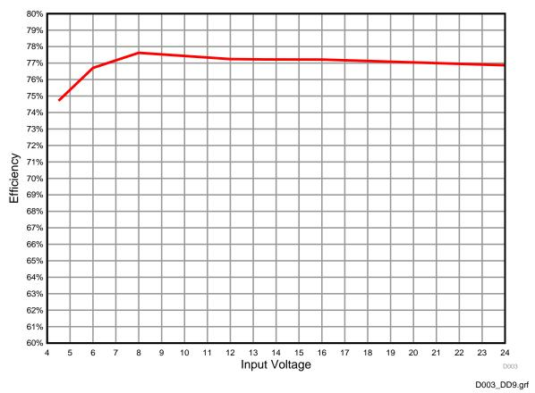
Figure 18. Total System Efficiency for Varying Input Voltage
