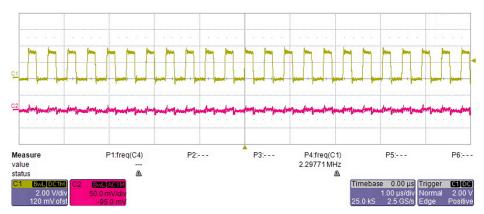
Figure 22. LM26420-Q1 Switch Node and Output Voltage Ripple, 1.2-V Output at Full Load
