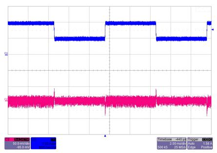
Figure 28. LM26420-Q1 50-100% Load Transient, 1.2 V
