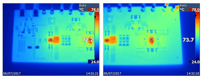
Figure 30. Thermal of LMS3655-Q1 at 5-A Load
