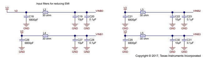
Figure 11. Input EMI Filter for Each Phase
