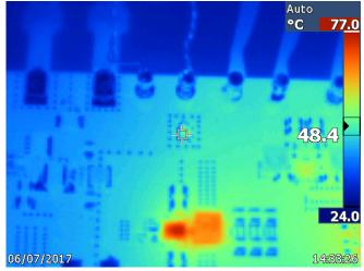
Figure 33. Thermal of LM2775 at 100-mA Load
