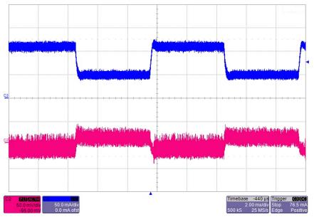
Figure 29. LM2775 50-100% Load Transient
