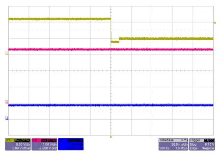
Figure 38. Cold Crank Down to 3.5 V, LP87561–Q1: 0.9 V at 10-A Output
