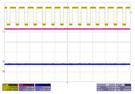
Figure 39. Warm Crank LP87561-Q1: 0.9 V at 10-A Output
