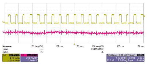
Figure 25. LP87561-Q1 Switch Node and Output Voltage Ripple, 0.9-V Output and Full Load
