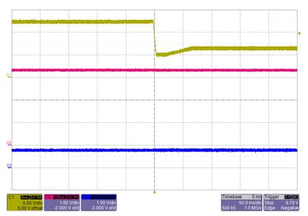
Figure 42. Start-Stop 50-ms Timescale, 0.9 V at 10-A Output
