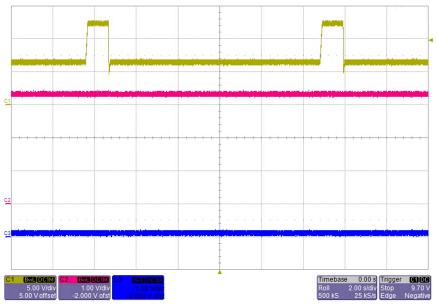
Figure 41. Start-Stop 5-s Timescale, 0.9 V at 10-A Output
