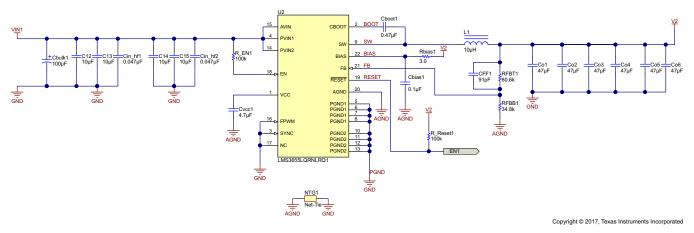
Figure 9. Wide Input Voltage Buck
