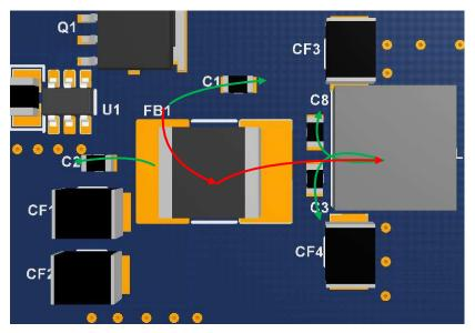
Figure 49. Input EMI Filter
