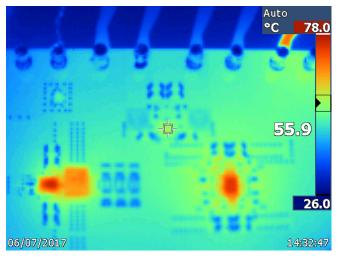
Figure 32. Thermal of LM26420-Q1 at 1 A for 1.8-V Rail and 2 A for 1.2-V Rail
