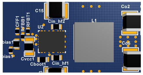
Figure 50. 3.3-V Supply Component Placement
