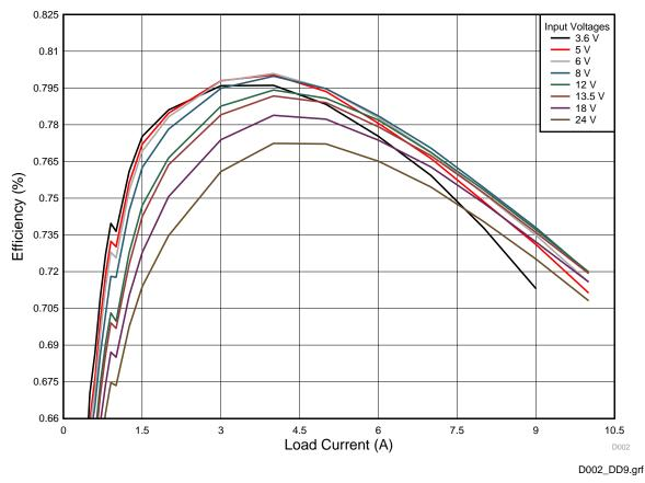
Figure 17. Two-Stage Efficiency
