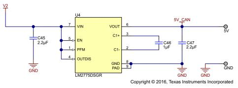
Figure 14. 5-V CAN Supply Schematic
