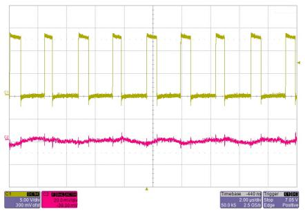
Figure 19. LMS3655-Q1 Switch Node and Output Voltage Ripple, 13.5-V Input at Full Load
