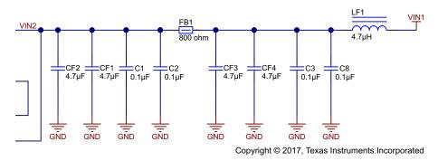
Figure 8. Input EMI Filter Schematic
