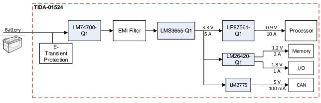
Figure 3. Power Solution for Single-Core-Voltage Application Processors
