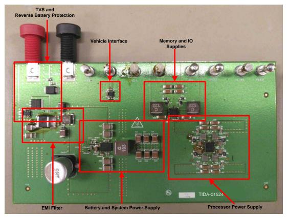
Figure 2. TIDA-01524 Subsystems Highlight
