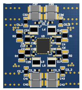
Figure 52. Core-Voltage Supply Component Placement—Top View
