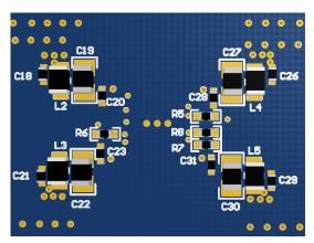
Figure 53. Core-Voltage Supply Passives Placement—Bottom View
