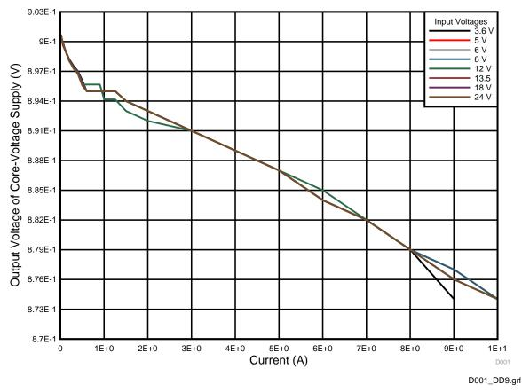
Figure 16. Load Regulation of Core-Voltage Supply
