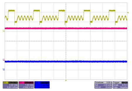
Figure 37. Cold Crank LP87561–Q1: 0.9 V at 10-A Output
