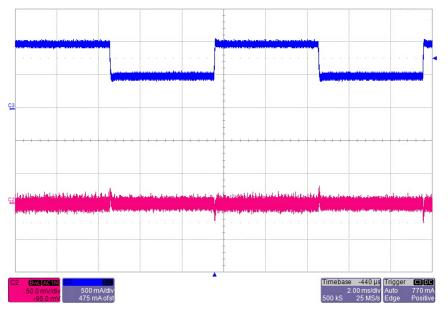
Figure 27. LM26420-Q1 50-100% Load Transient, 1.8 V
