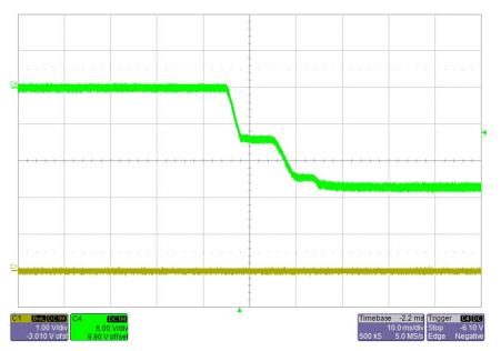
Figure 35. Transition to Reverse Voltage at Input
