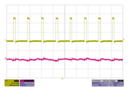
Figure 21. LMS3655-Q1 Switch Node and Output Voltage Ripple, 20-V Input at Full Load
