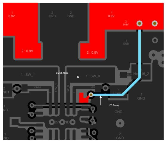
Figure 51. Routing Feedback Traces Around Switch Nodes
