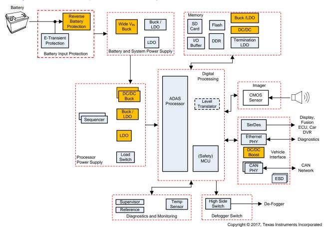
Figure 1. Example of Front Camera Block Diagram
