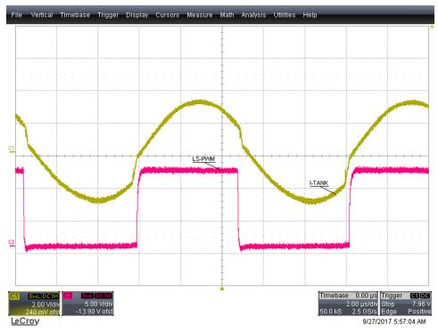
Figure 12. LLC Tank Current and Low-Side PWM
