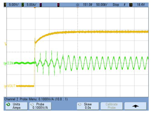
Figure 7. Startup Waveform at 230-V AC
