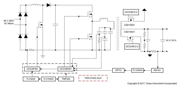
Figure 1. Block Diagram of TIDA-01494
