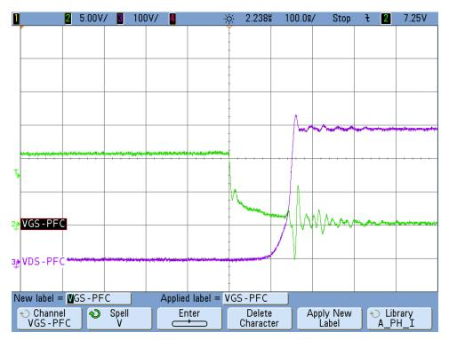
Figure 11. PFC MOSFET Turnoff Waveform
