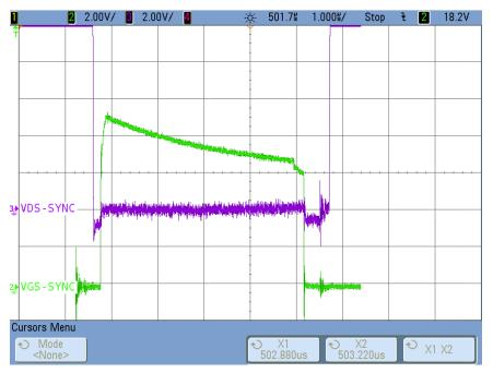
Figure 13. Synchronous MOSFET V<sub>DS</sub> and Proportion Gate Drive Signal
