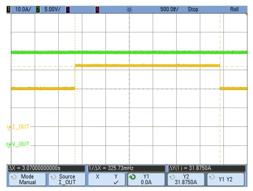
Figure 16. 720-W Peak Output Power Capability at 24-V Output
