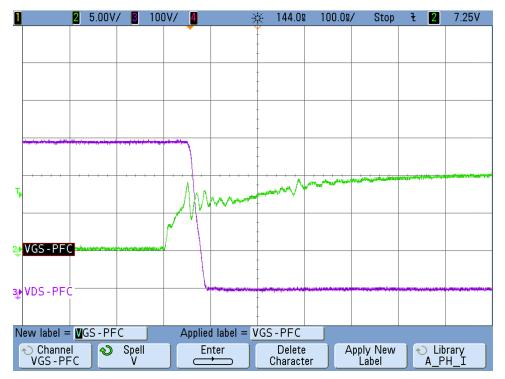
Figure 10. PFC MOSFET Turnon Waveform
