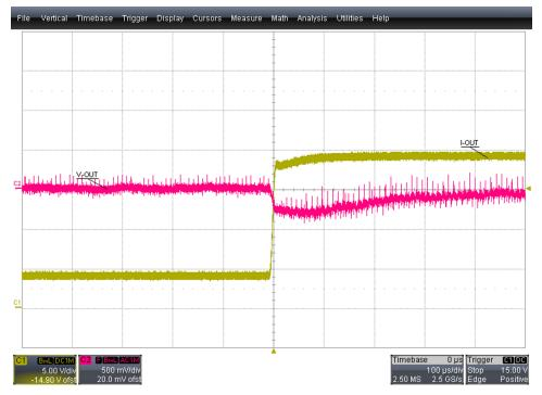
Figure 9. Transient Response at 24-V Output
