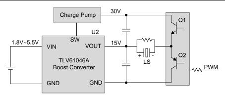
Figure 2: Block Diagram of ±15-V Driver Circuit
