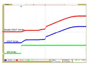
Figure 7: Startup at VIN=3.3V
