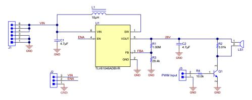
Figure 3: 28-V Rectangular Waveform Driver Circuit
