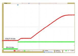
Figure 5: Startup at VIN=3.3V
