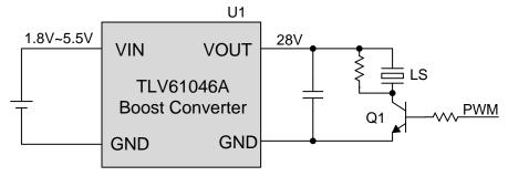
Figure 1: Block Diagram of the 28-V Driver Circuit
