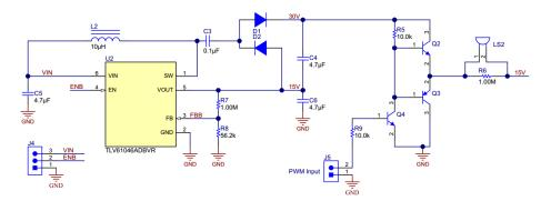
Figure 4: ±15-V Rectangular Waveform Driver Circuit
