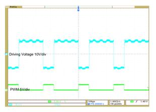
Figure 8: Operating Waveform with 4-KHz PWM
