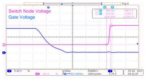
Figure 25. Turnon and Turnoff Times of IGBT at 250-V Bus Voltage Using IGBT CM100TX-24S With UCC5350MCD
