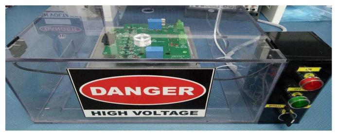
Figure 33. Image of Board Inside High-Voltage Safety Box
