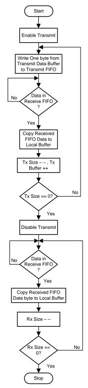
Figure 7. Transmit and Receive Flow Chart
