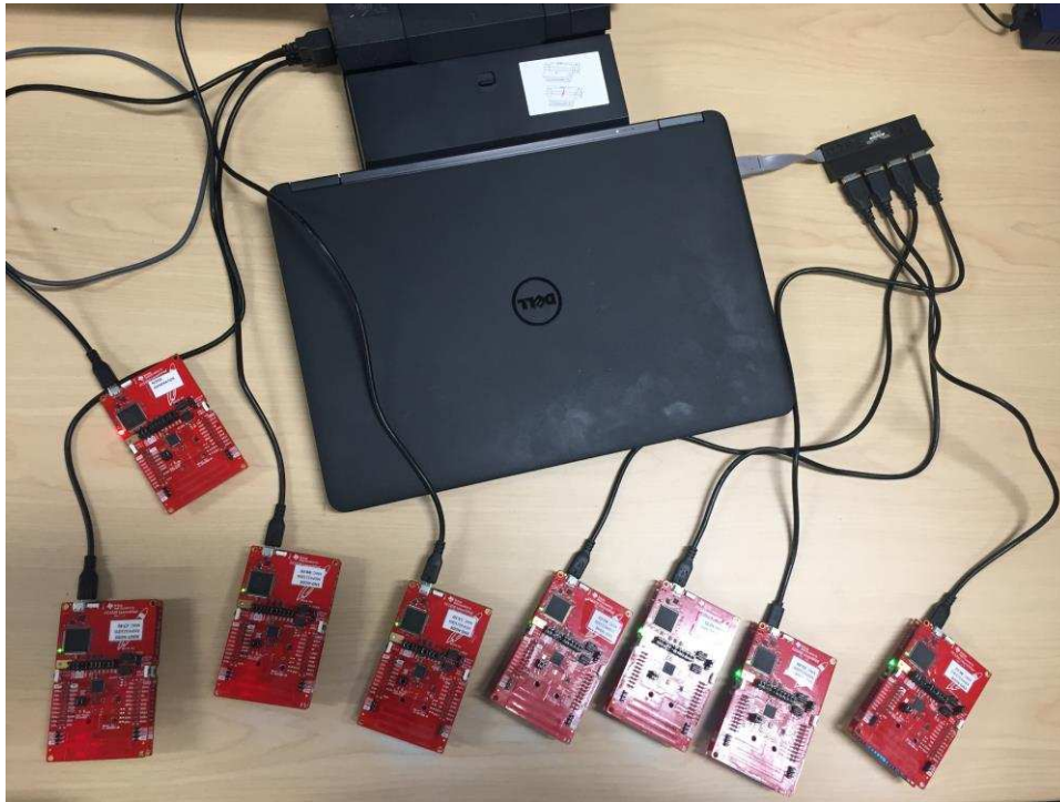
Figure 26. Multi-Hop Network Setup With Noise Generator
