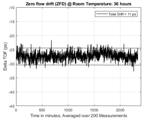
Figure 21. Zero-Flow Drift of DToF at Room Temperature
