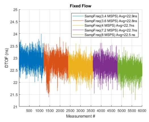
Figure 25. DToF of 1 GPM at Different Sampling Rates
