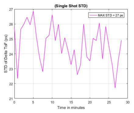
Figure 20. Single-Shot Standard Deviation at Room Temperature
