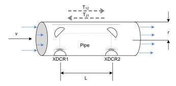
Figure 2. ToF in Flow Meter
