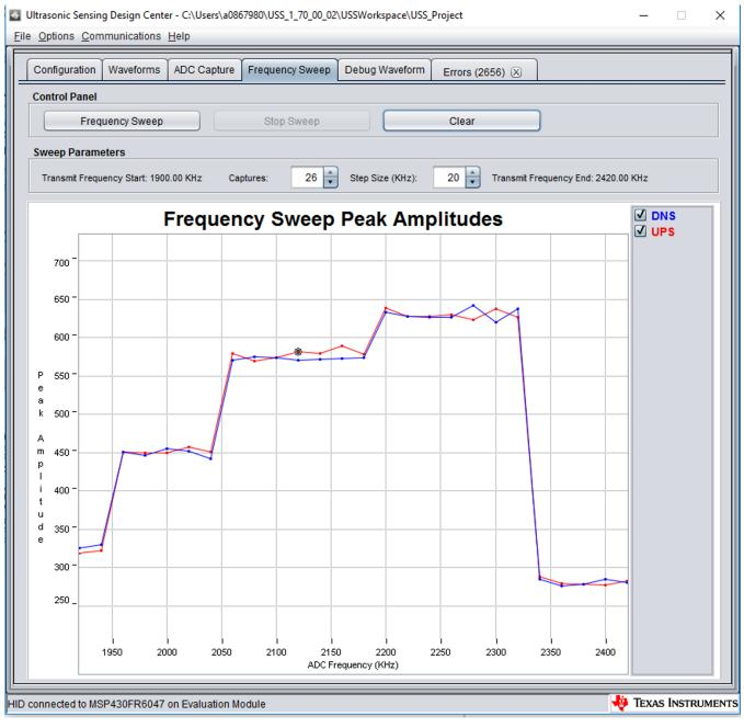
Figure 15. Frequency Response Test Results
