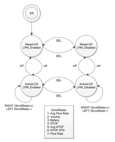
Figure 9. LCD and Buttons State Machine
