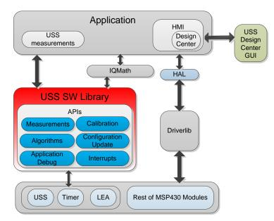
Figure 7. Software Architecture
