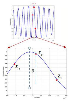
Figure 3. Interpolation Step for Differential ToF
