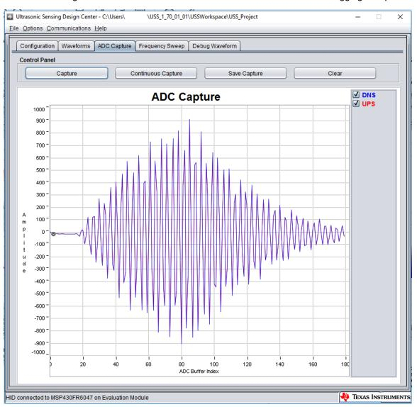
Figure 13. USS Design Center ADC Waveform Capture Window
