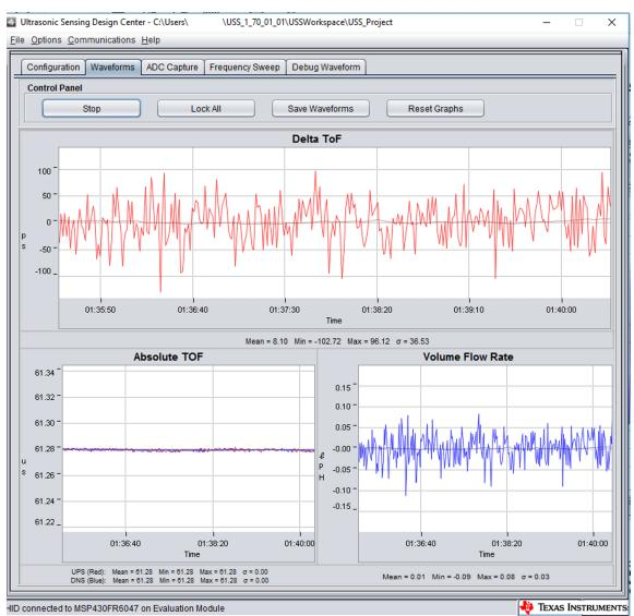
Figure 12. USS Design Center GUI Waveforms Window
