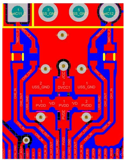
Figure 28. Layout Guidelines: Transducer Symmetric Traces
