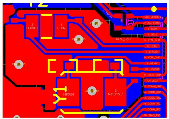
Figure 27. Layout Guidelines: Oscillator
