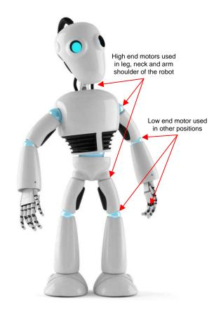
Figure 1. Typical Humanoid—Motor Drive Locations
