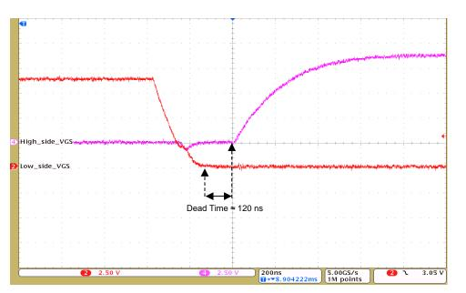
Figure 17. Dead Time at Trailing Edge of Low-Side V<sub>GS</sub>
