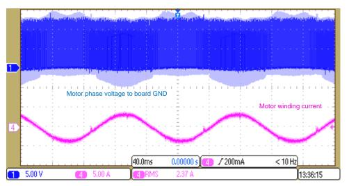
Figure 24. Load Test Results With Sinusoidal Control at 2.37-A $_{\rm RMS}$  Winding Current
