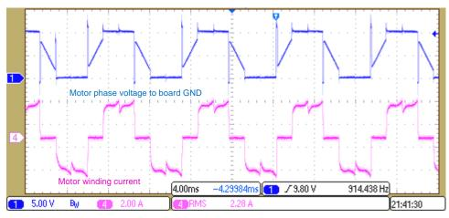
Figure 22. Load Test Results With Trapezoidal Control at 2.28-A<sub>RMS</sub> Winding Current, 100% Duty Cycle
