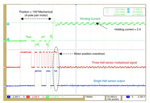
Figure 29. Test Results for Position Control at 105° Mechanical
