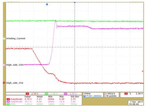
Figure 21. High-Side FET Turnoff: High-Side  $V_{\text{GS}}$  and  $V_{\text{DS}}$  at 2-A Winding Current
