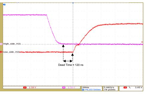
Figure 16. Dead Time at Rising Edge of Low-Side  $V_{\rm GS}$
