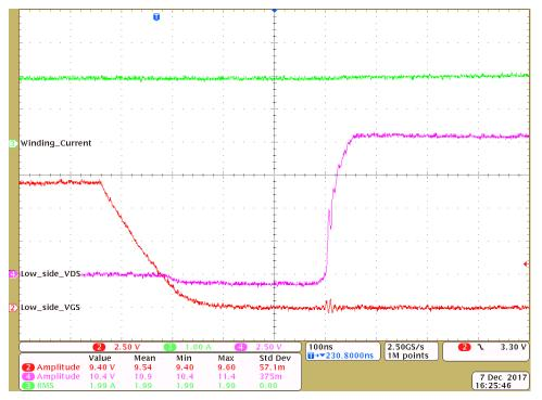
Figure 19. Low-Side FET Turnoff: Low-Side  $V_{\text{GS}}$  and  $V_{\text{DS}}$  at 2-A Winding Current
