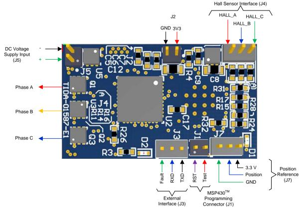
Three-pin connector J4: This connector interfaces hall senor position signal from the motor.
