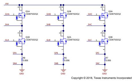
Figure 4. Schematic of Three-Phase Inverter
