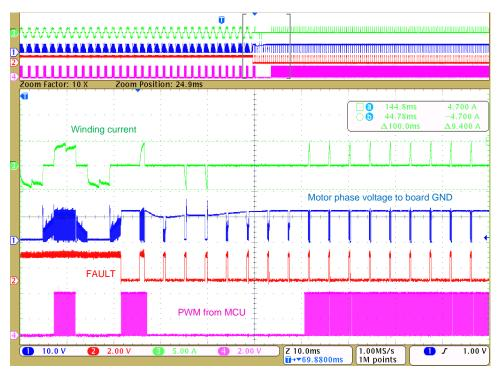
Figure 27. Overcurrent Protection With MOSFET V<sub>DS</sub> Monitoring
