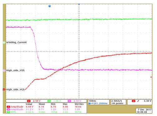
Figure 20. High-Side FET Turnon: High-Side  $V_{\rm GS}$  and  $V_{\rm DS}$  at 2-A Winding Current
