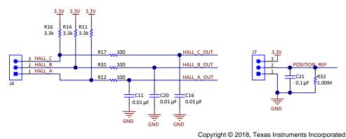
Figure 8. Schematic of Position Feedback
