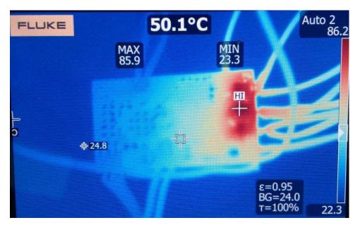
Figure 25. Thermal Image of Board With Sinusoidal Control at 2.37-A<sub>RMS</sub> Winding Current
