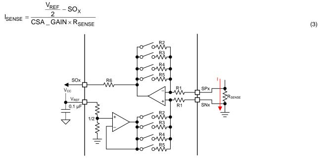
Figure 6. DRV8304 Current Sense Amplifier
