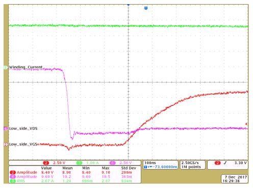
Figure 18. Low-Side FET Turnon: Low-Side  $V_{\rm GS}$  and  $V_{\rm DS}$  at 2-A Winding Current
