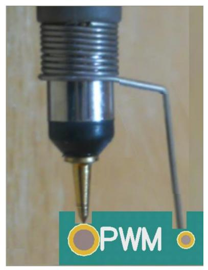
Figure 9. Low Parasitic Measurement Setup
