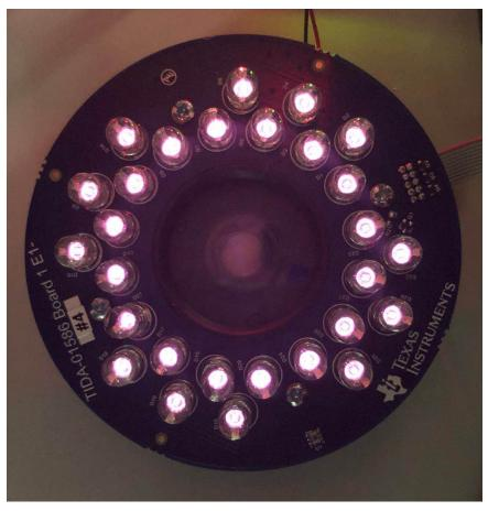
Figure 34. Ballasting Effect for IR LEDs Uniform Illumination
