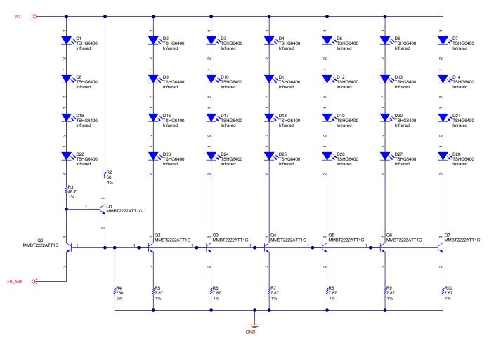
Figure 8. IR LED Arrays With Ballasting
