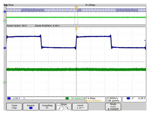
Figure 36. PWM Duty Cycle at 50% Buck LED Driver
