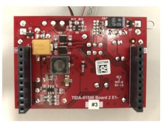
Figure 18. Power and Control Board (Board-2) Back Side
