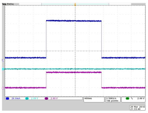
Figure 44. Current Consumption Difference in Sleep Current and Coil Current
