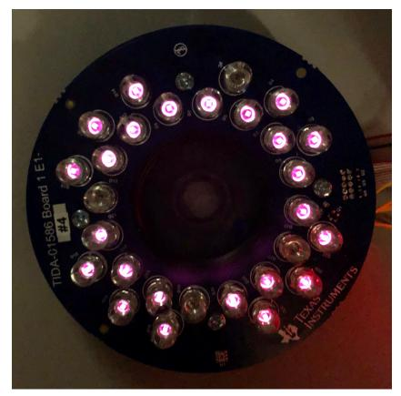
Figure 33. IR LEDs illumination Without Ballasting
