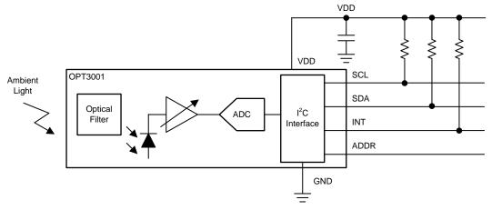
Figure 6. OPT3001 Functional Block Diagram
