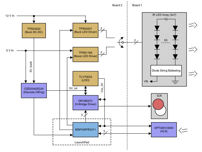
Figure 1. TIDA-01586 Block Diagram
