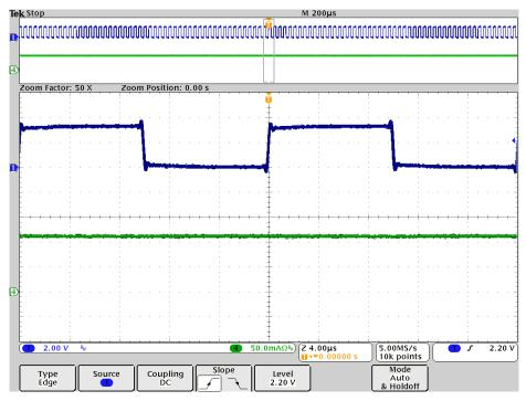
Figure 40. PWM Duty Cycle at 50% for Boost LED Driver
