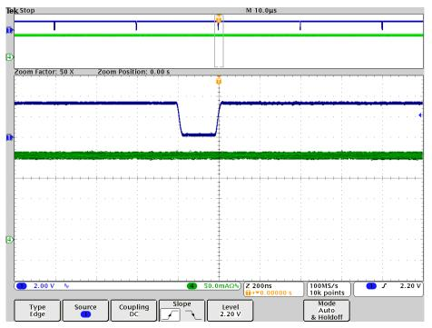
Figure 37. PWM Duty Cycle at 99% Buck LED Driver
