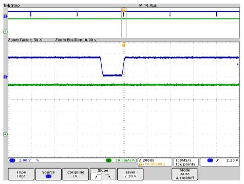
Figure 41. PWM Duty Cycle at 99% for Boost LED Driver
