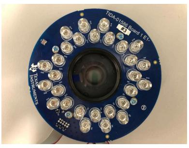
Figure 19. IR LED Array and ALS Board (Board-1)
