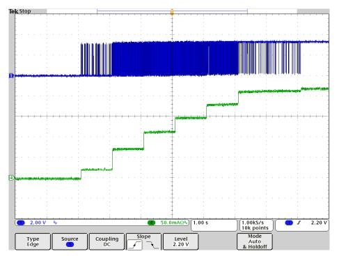
Figure 42. Boost LED Driver From Disable to 100% Duty Cycle
