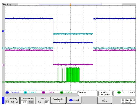
Figure 43. Bidirectional Current Control Using the DRV8837C
