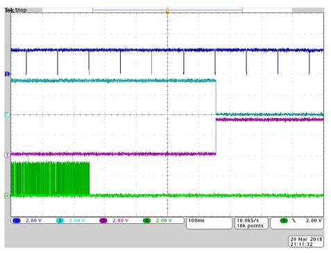
Figure 32. Ambient Light Level From LED Disabled Area to ICR Closed Area
