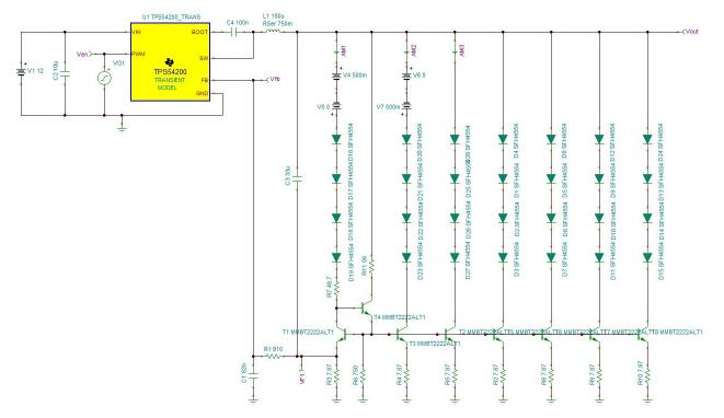
Figure 11. Simulation Circuit With Channel Ballasting
