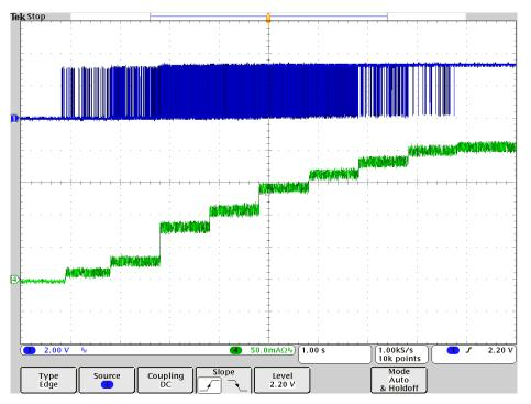
Figure 38. Buck LED Driver From Disable to 100% Duty Cycle
