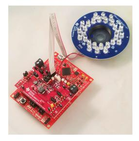
IR LED Illumination and ICR Control Reference Design for IP Network Cameras With Day/Night Vision Copyright © 2018, Texas Instruments Incorporated
