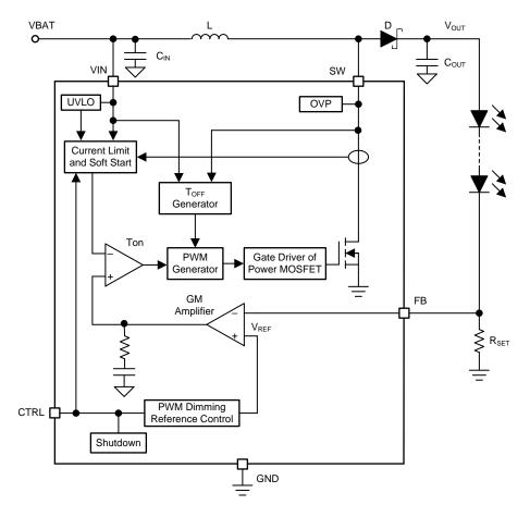
Figure 4. TPS61169 Functional Block Diagram
