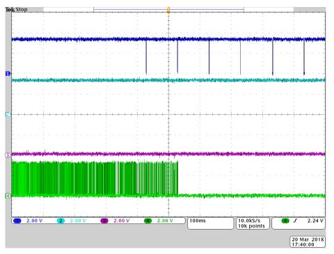
Figure 26. Ambient Light Level From LED Dimming Area to LED Disabled Area
