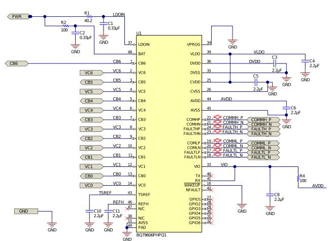
Figure 23. BQ79606A-Q1 Schematic
