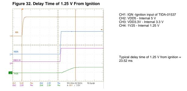
Performance of input power sequence is well within the design specification. It is in line with the description explained in Section 2.3.1.
