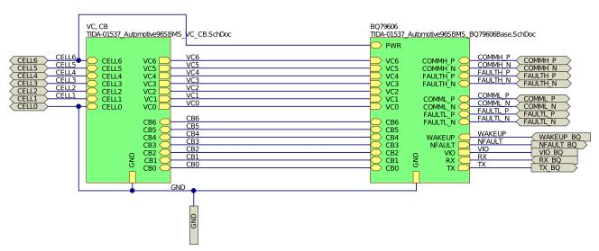
Figure 21. BQ79606A-Q1 Interface Block Diagram
