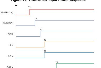
Figure 12. TIDA-01537 Input Power Sequence
