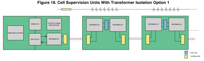
Transformer Isolation for board-to-board in Figure 18 helps in utilizing the BQ79606A-Q1 device for high-voltage measurements. The BQ79606A-Q1 on the first board (battery control unit) is isolated to the controller, which allows for high-voltage measurements. Transformer isolation is used for daisy-chain communication between the two cell supervision units.
