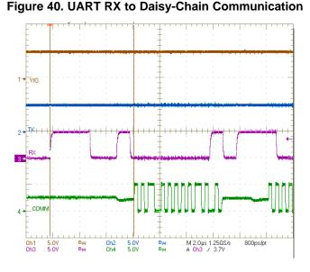
CH1: VIO - Interface to host BQ79606A-Q1 CH2: TX - UART of BQ79606A-Q1 CH3: RX - UART of BQ79606A-Q1 CH4: COMM - North COMM of host BQ79606A-Q1
