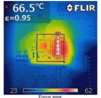
BQ79606A-Q1 + Balancing Resistors
