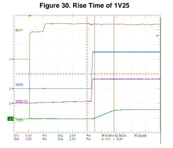
CH1: BATT -12-V battery voltage CH2: VDD5 - Internal 5 V CH3: VDD3.3V - Internal 3.3 V CH4: 1V25 - Internal 1.25 V
