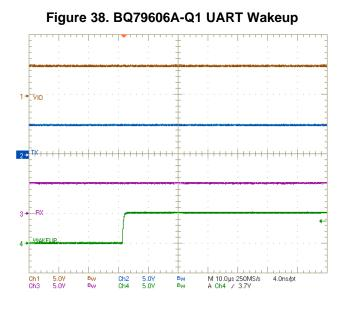
CH1: VIO - Interface to host BQ79606A-Q1 CH2: TX - UART of BQ79606A-Q1 CH3: RX - UART of BQ79606A-Q1 CH4: WAKEUP - BQ79606A-Q1
