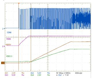
CH1: VDD5V - Internal 5 V CH2: SDN6 -TPS65381-Q1 CH3:VDD6 -TPS65381-Q1 CH4: VDD3.3 - Internal 3.3 V
