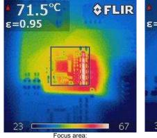
BQ79606A-Q1 + Balancing Resistors
