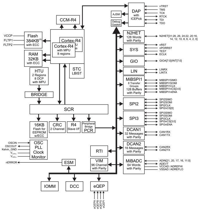
Figure 4. TMS570LS0432 Block Diagram
