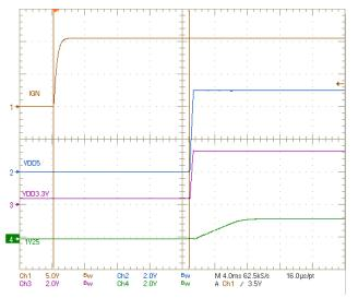
CH1: IGN -Ignition input of TIDA-01537 CH2: VDD5 - Internal 5 V CH3: VDD3.3V - Internal 3.3 V CH4: 1V25 - Internal 1.25 V
