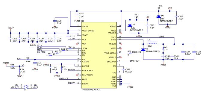
Switch S1 is used to emulate the ignition behavior onboard. The CAN wakup feature is not used in the TIDA-01537 design.
