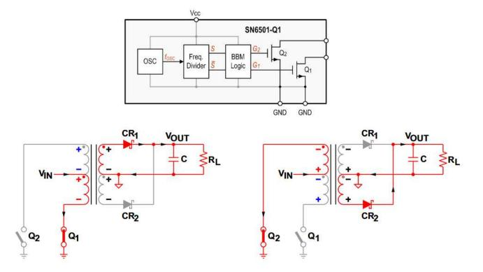
Figure 9. SN6501-Q1 Functional Block Diagram
