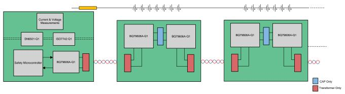
Figure 19. Cell Supervision Units With Transformer Isolation Option 2
