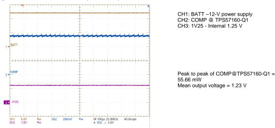
Figure 34. TPS57610-Q1 Comp and Output Behavior
