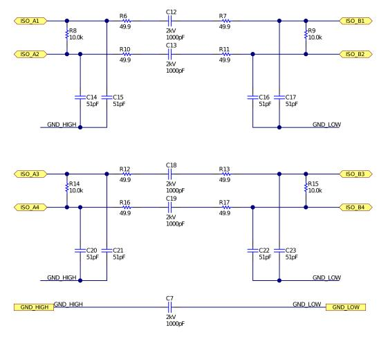
Figure 24. Capacitive Isolation for BQ79606A-Q1
