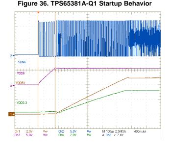
CH1: VDD5V - Internal 5 V CH2: SDN6 -TPS65381-Q1 CH3:VDD6 -TPS65381-Q1 CH4: VDD3.3 - Internal 3.3 V
