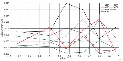
The leakage current of the VCx and CBx pins is low in all operating modes of the BQ79606A-Q1 device.
