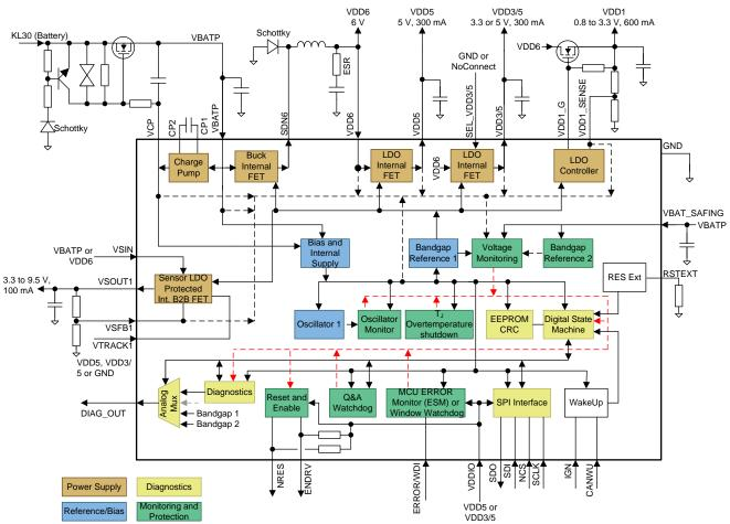
Figure 5. TPS65381A-Q1 Block Diagram
