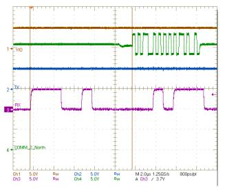
CH1: VIO - Interface to host BQ79606A-Q1 CH2: TX - UART of BQ79606A-Q1 CH3: RX - UART of BQ79606A-Q1 CH4: COMM 2 North - North COMM of second BQ79606A-Q1
