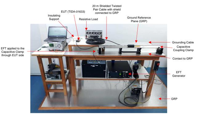
Figure 65. Lab EFT Test Setup
