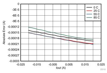
Figure 39. Measurement Error vs Output Current at Different Temperatures
