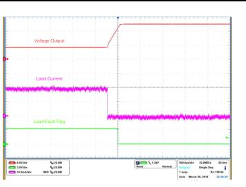
Figure 50. Open Load Fault Detection - Initial lout is +20 mA
