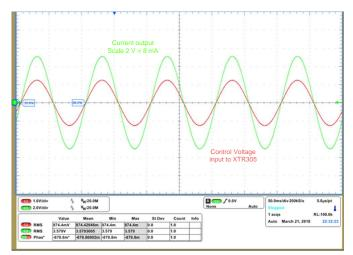
Figure 43. Input Sine Voltage and Output Sine Current at 10 Hz
