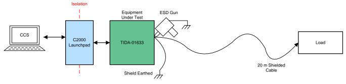
Figure 60. ESD Test Setup Diagram
