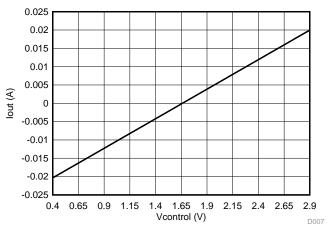
Figure 36. Current Output Transfer Function
