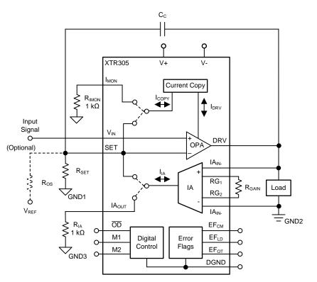
Figure 3. XTR305 Based Fully Integrated Solution
