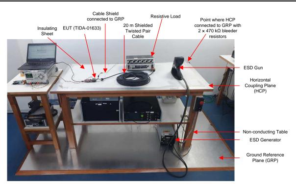
Figure 61. Lab Test Setup
