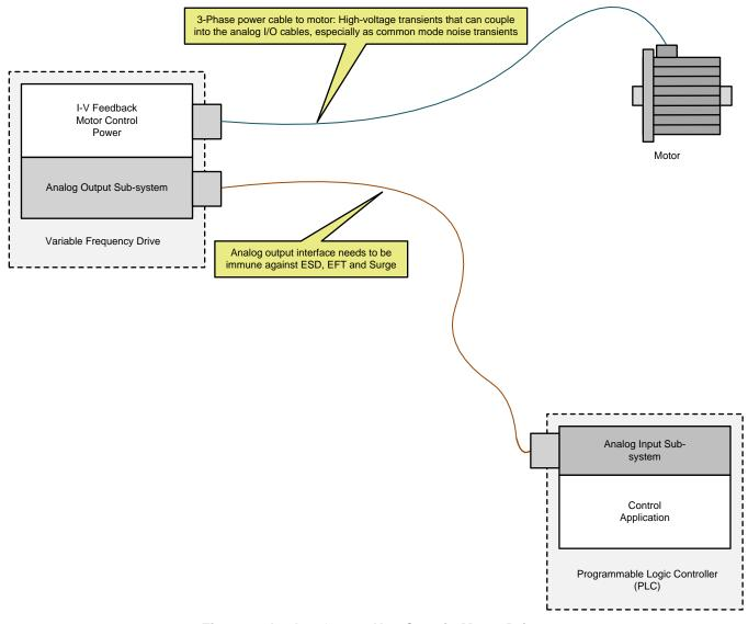
Figure 1. Analog Output Use Case in Motor Drives
