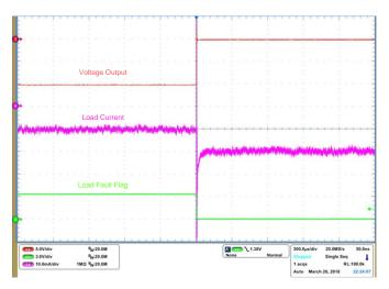
Figure 49. Load Short Detection - Initial Vout is -10 V
