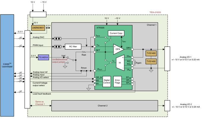
Figure 4. TIDA-01633 Block Diagram
