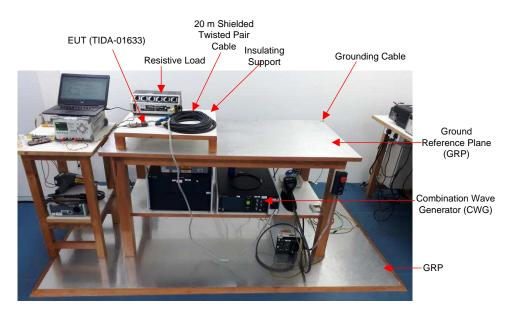
Figure 67. Lab Surge Test Setup
