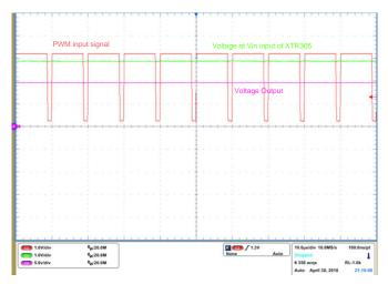
Figure 34. Voltage Output at 87.87% Duty Cycle
