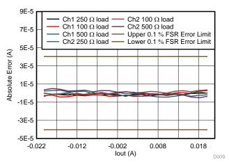
Figure 38. 2-Point Calibrated Measurement Error vs Output Current at Different Loads
