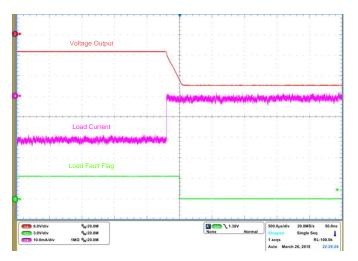
Figure 51. Open Load Fault Detection - Initial lout is -20 mA
