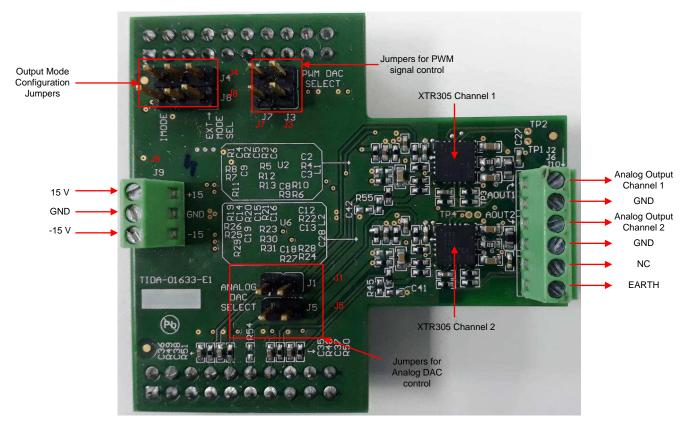
Figure 20. Top View of TIDA-01633
