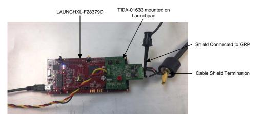
Figure 62. EUT (TIDA-01633) Connections
