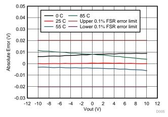
Figure 27. 2-Point Calibrated Measurement Error vs Output Voltage at Different Temperatures
