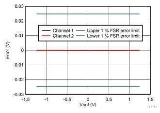
Figure 55. 2-Point Calibrated Measurement Error vs Analog Input Voltage
