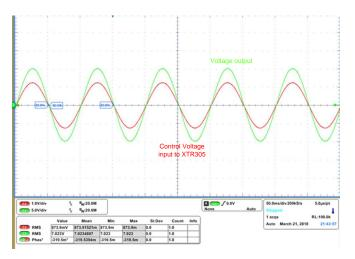
Figure 30. Input and Output Sine Voltages at 10 Hz
