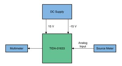
Figure 52. Test Setup for Analog Input Mode
