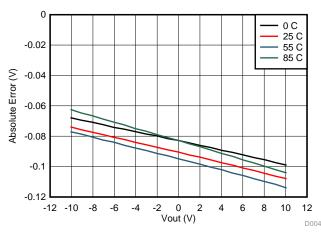
Figure 26. Measurement Error vs Output Voltage at Different Temperatures
