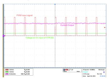
Figure 45. Current Output at 12.12% Duty Cycle
