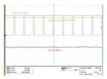
Figure 47. Current Output at 87.87% Duty Cycle
