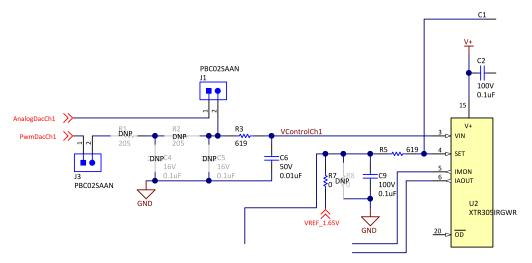
Figure 12. Analog DAC Based Control of Analog Output
