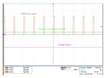
Figure 32. Voltage Output at 12.12% Duty Cycle
