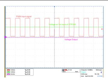
Figure 33. Voltage Output at 50% Duty Cycle
