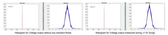
Figure 59. Histogram Before EMC Transients and During EMC Transient
