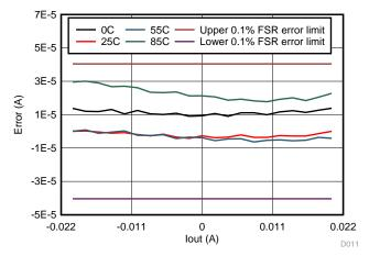
Figure 40. 2-Point Calibrated Measurement Error vs Output Current at Different Temperatures
