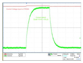
Figure 41. Small Signal Step Response
