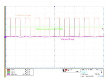
Figure 46. Current Output at 50% Duty Cycle
