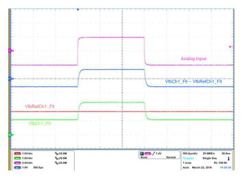
Figure 57. Large Signal Step Response
