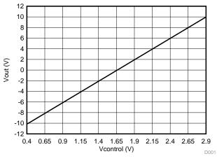
Figure 23. Voltage Output Transfer Function
