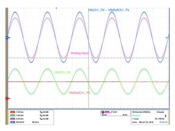
Figure 58. Sine Input and Output at 10 Hz
