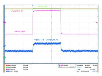
Figure 56. Small Signal Step Response
