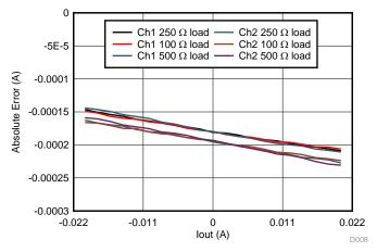
Figure 37. Uncalibrated Measurement Error vs Output Current at Different Loads
