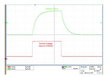
Figure 29. Large Signal Step Response
