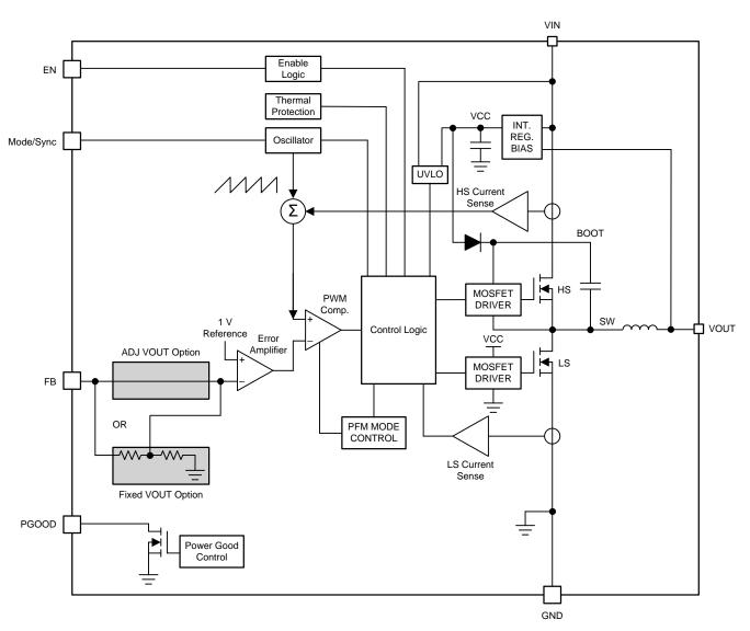
Figure 8. Functional Block of LMZM23601
