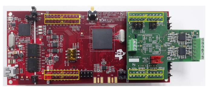
Figure 21. Launchpad Interface to TIDA-01633
