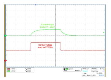
Figure 42. Large Signal Step Response
