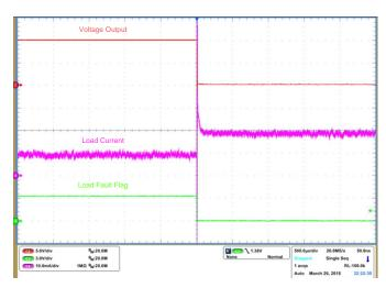
Figure 48. Load Short Detection - Initial Vout is +10 V
