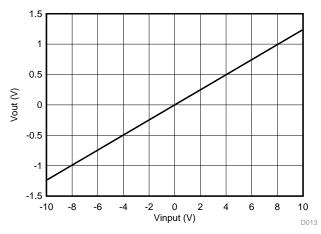
Figure 53. Analog Input Transfer Function
