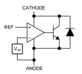
Figure 7. Functional Block of TLV431A
