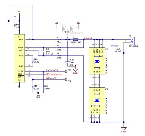
Figure 10. Output EMC Protection Components
