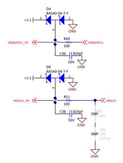
Figure 15. RC Filters on ADC Input
