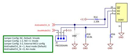
Figure 11. Analog Output Pin Mode Selection
