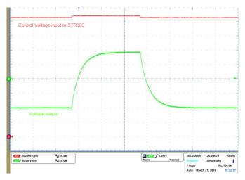
Figure 28. Small Signal Step Response
