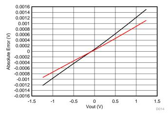
Figure 54. Uncalibrated Measurement Error vs Analog Input Voltage
