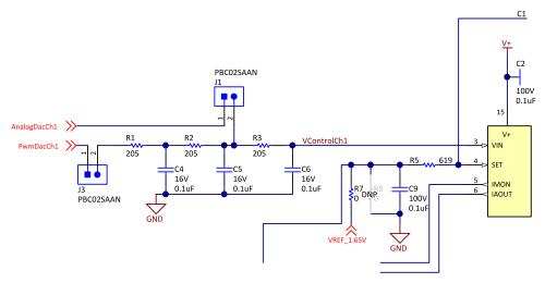
Figure 13. PWM Control of Analog Output
