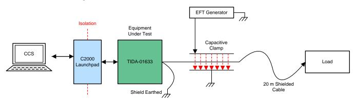
Figure 64. EFT Test Setup Diagram
