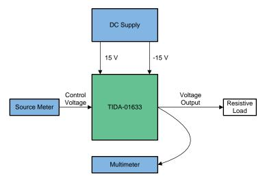
Figure 22. Test Setup for Voltage Output Mode
