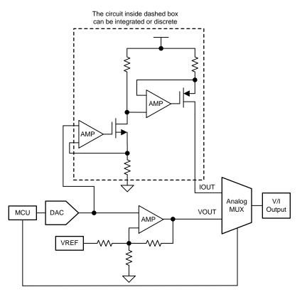
Figure 2. Discrete and Partially Discrete Analog Output Implementation Example
