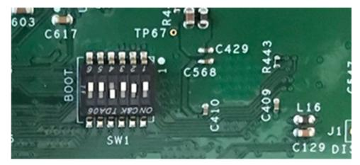
Figure 9. Boot Mode Switch SW1 Settings
