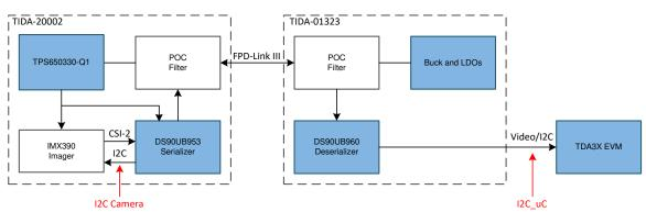
Figure 10. Setup for Monitoring I<sup>2</sup>C Transactions
