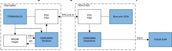
Figure 7. Block Diagram of Characterization Test Setup
