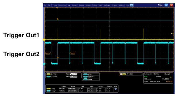
Figure 9. Scope plots of Trigger Out1 and Trigger Out2 (24-bit Monochrome)
