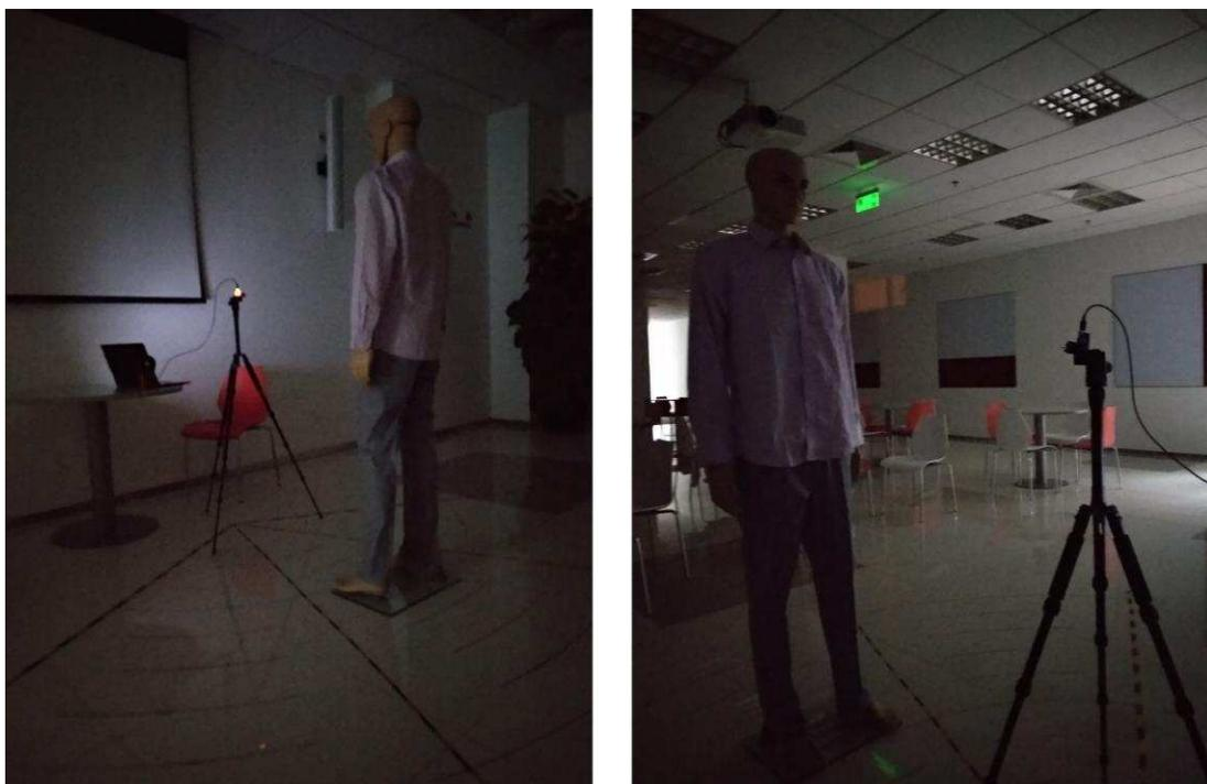
For the darkness operation, only model B is chosen and placed in Zone 2 for the test. Comparing with the same position of Scene 1, sensor performance under darkness operation can be observed and effects of low ambient light can be concluded. In Figure 48, the red line shows the test results comparing with gray line which is sensor performance in Scene 1.
