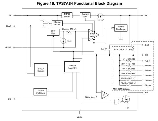
The TPS7A84 is a low-noise (4.4  $\mu$ V<sub>RMS</sub>), low-dropout linear regulator (LDO) capable of sourcing 3 A with only 180 mV of maximum dropout. The device output voltage is pin-programmable from 0.8 V to 3.95 V and adjustable from 0.8 V to 5.0 V using an external resistor divider.
