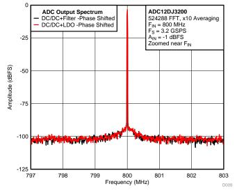
Figure 25. ADC Output, Filter vs LDO (Near DC)
