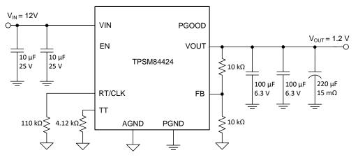
Figure 7. TPSM84424 Circuit Diagram
