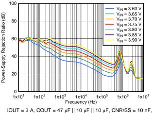
$1001 = 3 \text{ A}, \text{ COUT} = 47 \ \mu\text{F} \parallel 10 \ \mu\text{F} \parallel 10 \ \mu\text{F}, \text{ CNR/SS} = 10 \ \text{nF}, \text{CFF} = 10 \ \text{nF}$
