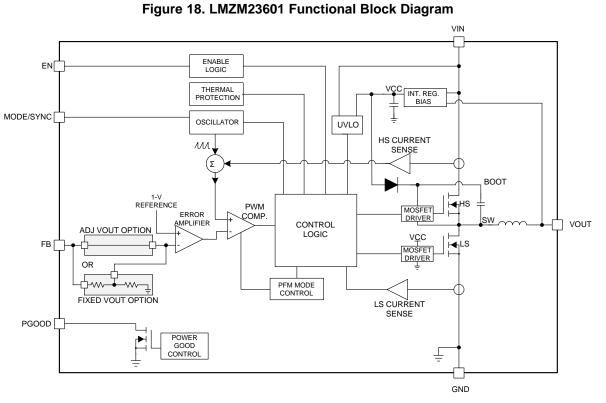
The LMZM23601 device is an integrated-inductor power module, that is specifically designed for spaceconstrained industrial applications. It is used in this design to bring down the 12-V input voltage to  $\pm 2.5$  V. It is available in two fixed output voltage options of 5-V and 3.3-V, and an adjustable (ADJ) output voltage option supporting a 2.5-V to 15-V range. The LMZM23601 has an input voltage range of 4-V to 36-V and can deliver up to 1000-mA of output current.
