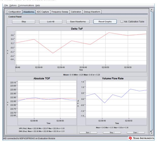
Figure 3-8. USS Design Center GUI Waveforms Window
