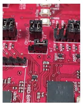
Figure 3-2. USB (eZ-FET) Power Jumper Configuration
