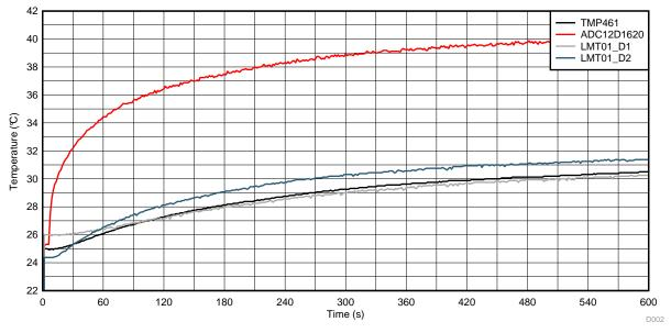
Figure 5. TSW12D1620EVM-CVAL Board Temperatures Operating at 4 W
