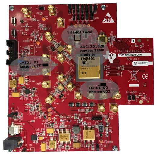
Figure 4. TSW12D1620EVM-CVAL Temperature Sensor Locations
