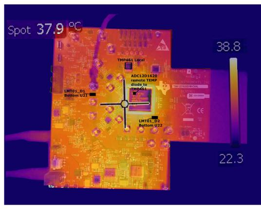
Figure 7. TSW12D1620 Thermal Infra-Red Composite Board Image
