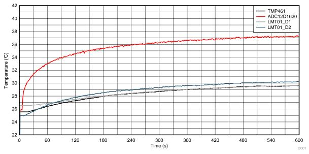
Figure 6. TSW12D1620EVM-CVAL Board Temperatures Operating at 2 W
