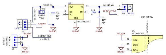
C11 is the input bypass capacitor, C10 acts as output capacitor of the ISO LDO. The ISO LDO is equipped with a dedicated testpoint and one dedicated header, enabling probing of dedicated signals:
