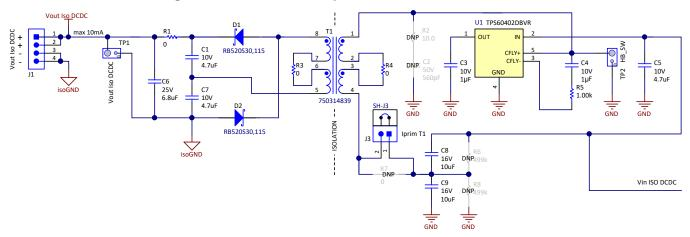
Figure 17. TIDA-010018: Implementation of the ISO DC/DC
