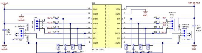
This reference design features one transmit channel and three receive channels on the isolated side and three transmit- and one receive-channel on the non-isolated side.
