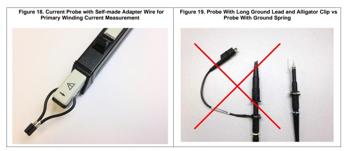
The reference design contains test points (TP) for all the different circuit blocks to simplify the evaluation of the board. To modify the probe, remove the probe tip cover. In addition, the ground lead and alligator clip must be replaced by a ground spring as Figure 19 shows. The modified probes fit directly into the test points (TP). The small ground spring significantly reduces the noise, which can couple otherwise into the long ground lead of a standard probe configuration.
