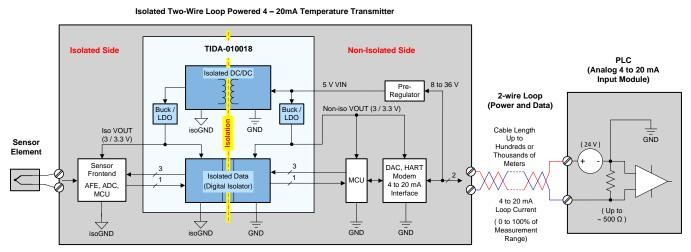
Figure 1. TIDA-010018 in Isolated Two-Wire Loop Powered 4- to 20-mA System
