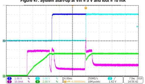
Figure 47. System Start-up at Vin = 5 V and lout = 10 mA
