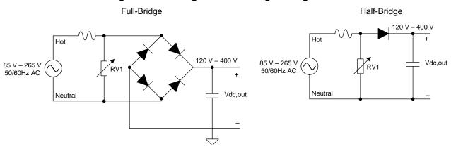
Figure 5. Full-Bridge and Half-Bridge Configuration
