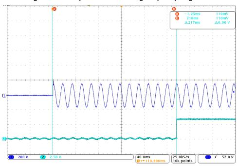
Figure 14. Startup Time for Half-bridge Cap-Drop Regulator
