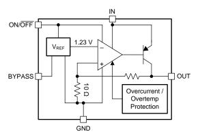
Figure 4. LP2992 Functional Block Diagram
