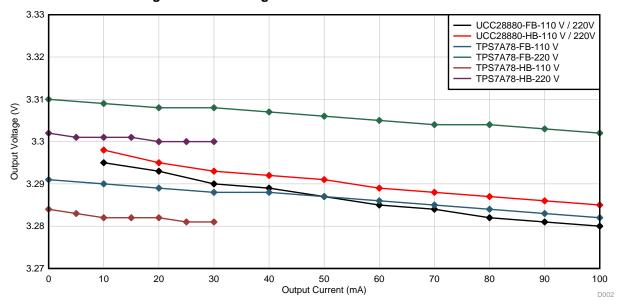
Figure 13. Load Regulation for Different Architectures
