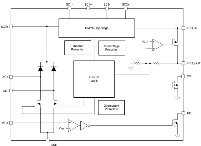
Figure 2. TPS7A78 Functional Block Diagram
