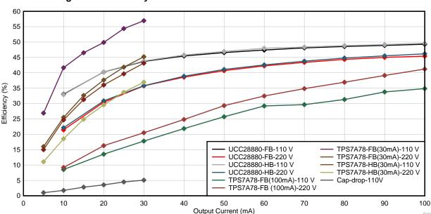
Figure 12. Efficiency Across Load Variations for Different Architectures
