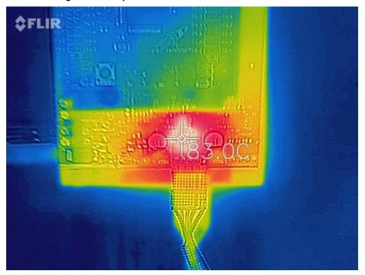
Figure 14. Temperature on DRV8889-Q1 With 1-A Current
