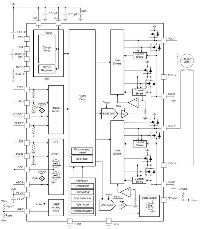
Figure 2. DRV8889-Q1 Functional Block Diagram
