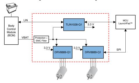
Figure 1. TIDA-020026 Block Diagram
