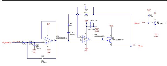
Figure 2-10. Electrochromic Mirror Driver Circuit
