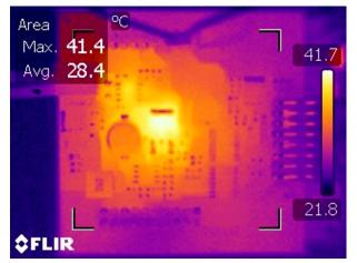
Figure 3-11. Thermal Image of PCB While Driving the Electrochromic Mirror
