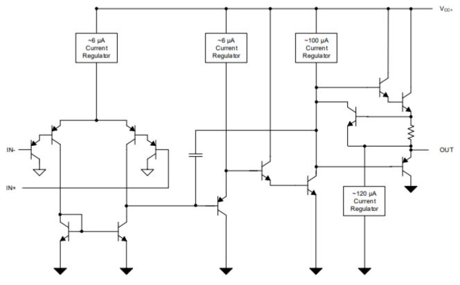
Figure 2-5. LM2904B-Q1 Block Diagram
