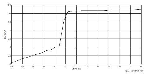
Figure 3-7. Input Voltage vs Input Current Graph
