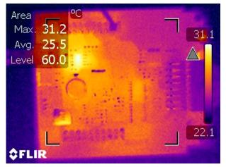
Figure 3-8. Reference Thermal Image of PCB
