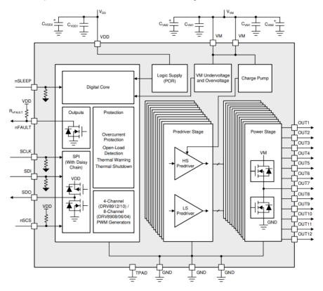
Figure 2-2. DRV8906-Q1 Block Diagram
