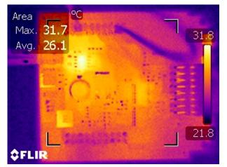
Figure 3-10. Thermal Image of PCB While Driving the Fold Motor
