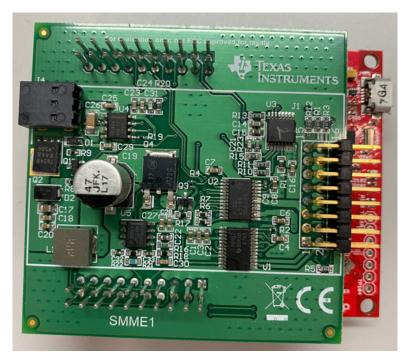
Figure 3-4. Image of TIDA-020027 Connected to MSP-EXP430F5529LP LaunchPad™
