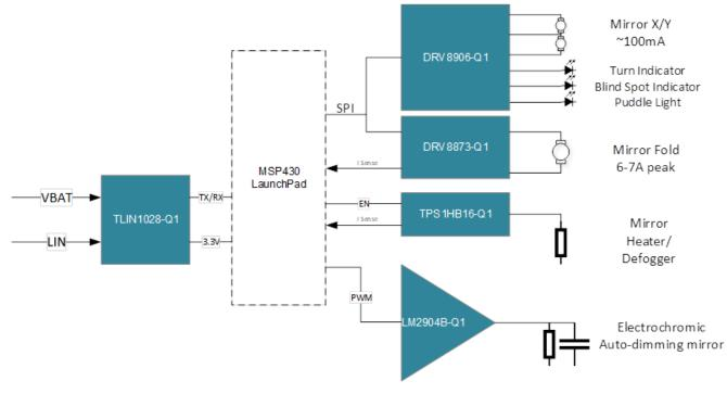
Figure 2-1. TIDA-020027 Block Diagram
