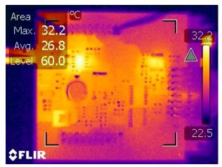
Figure 3-9. Thermal Image of PCB While Driving the Mirror Heater
