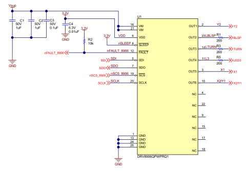
Figure 2-7. DRV8906-Q1 Configuration Schematic
