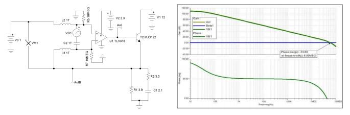
Figure 2-11. TINA-TI™ Stability Analysis of EC Mirror Driver Without Compensation
