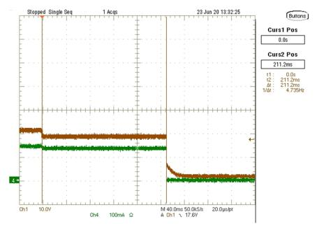
Figure 3-14. Highbeam/Lowbeam LED Short
