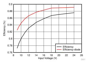
Figure 3-18. TIDA-050040 Full Load Efficiency
