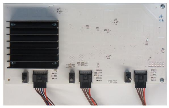
Figure 3-4. LED Load Board Bottom
