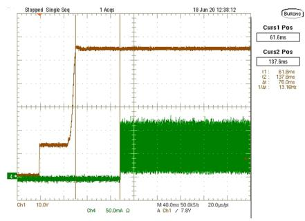
Figure 3-6. Highbeam/Lowbeam Turn on Delay
