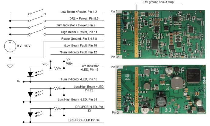
Figure 3-1. TIDA-50040 Test Connections for efficiency measurements, turn-on, turn-off delays and steady state operation
