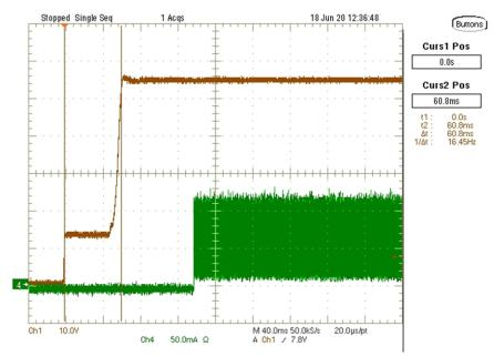
Figure 3-5. Boost Turn on Delay
