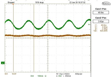
Figure 3-11. Turn Indicator Output Voltage and Current
