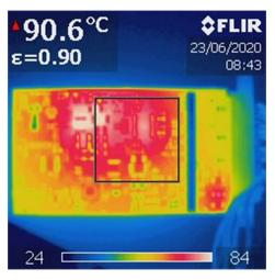
Figure 3-25. Top Side Thermal Image Highbeam/Lowbeam at 30W, Turn Indicator at 7.5W average
