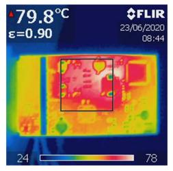
Figure 3-26. Bottom Side Thermal Image Highbeam/Lowbeam at 30W, Turn Indicator at 7.5W average
