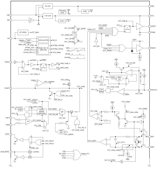
Figure 2-2. TPS92682-Q1 Functional Block Diagram
