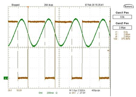
Figure 3-7. Highbeam/Lowbeam Switch Node and Ripple Current
