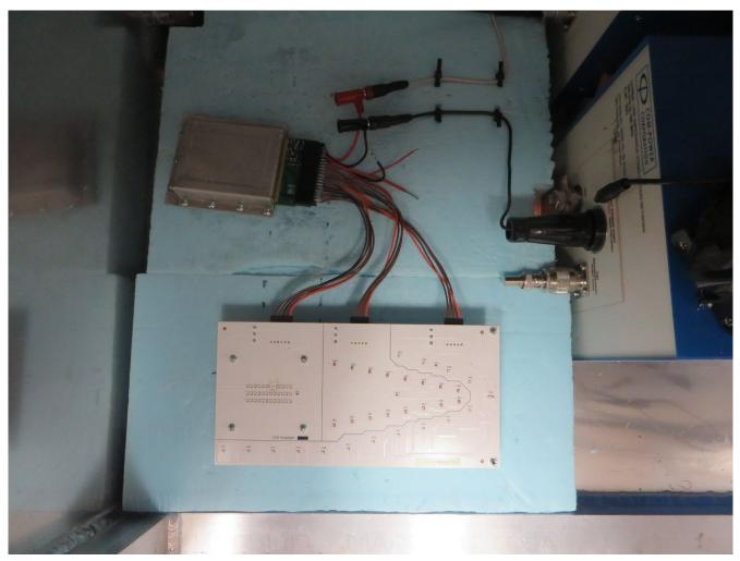
Figure 3-2. CISPR 25 Class 5 test setup
