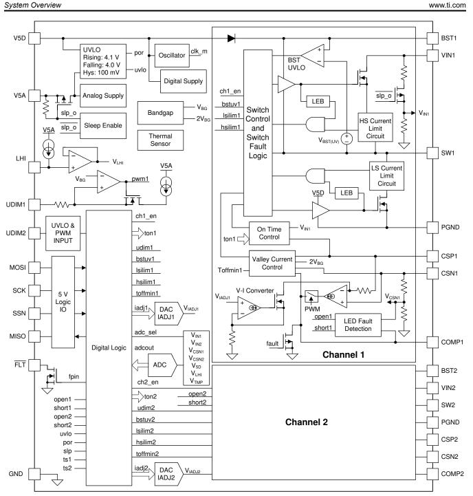
Figure 2-3. TPS92520-Q1 Functional Block Diagram
