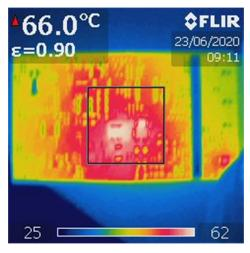
Figure 3-23. Top Side Thermal Image DRL at 15W
