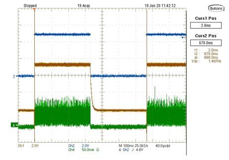
1.5 Hz Turn Indicator input (blue), Turn Indicator output (yellow) and current (green).
