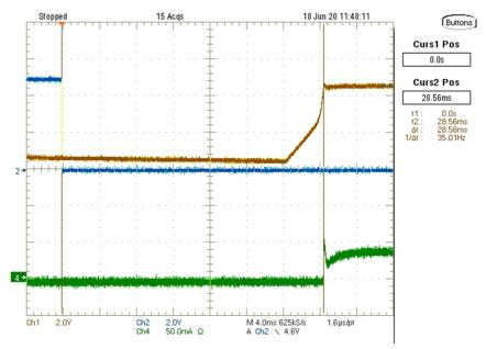
Figure 3-12. Daytime Running Light Turn-on Delay
