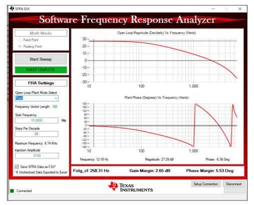
Figure 3-5. Plant Frequency Response
