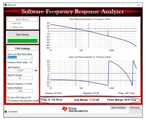
Figure 3-8. CC Mode Frequency Response
