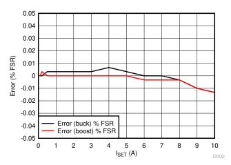
Figure 3-11. Constant-Current Control Accuracy ADS131M08 Feedback
