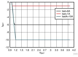
Figure 3-15. Discharge Mode CC to CV Transition
