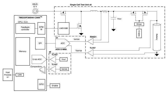
Figure 2-1. Digital Control Battery Tester
