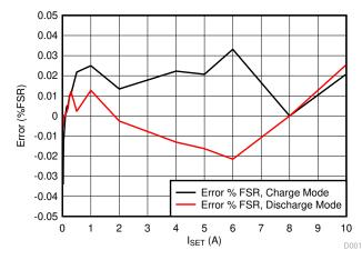
Figure 3-12. Constant-Current Control Accuracy 12-bit ADC Feedback
