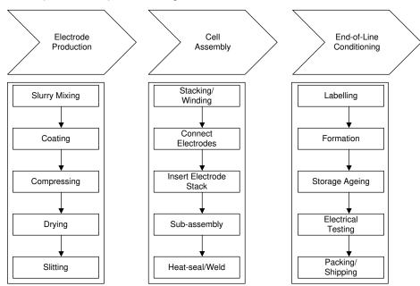
Figure 1-1. Simplified Li-Ion Battery Manufacturing Process
