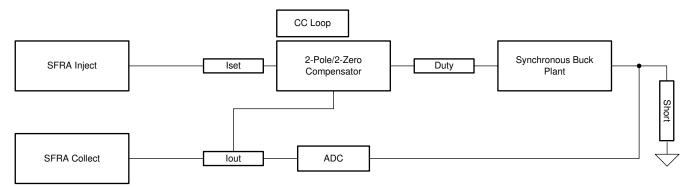
Figure 3-7. SFRA Setup Closed-Loop CC Mode
