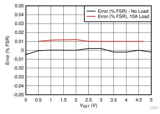
Figure 3-13. Constant-Voltage Control Accuracy
