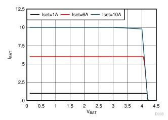
Figure 3-14. Charge Mode CC to CV Transition
