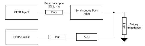
Figure 3-4. SFRA Setup for Plant Model Extraction
