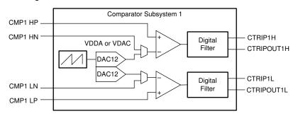
Figure 2-5. TMS320F280049 Comparator Subsystem
