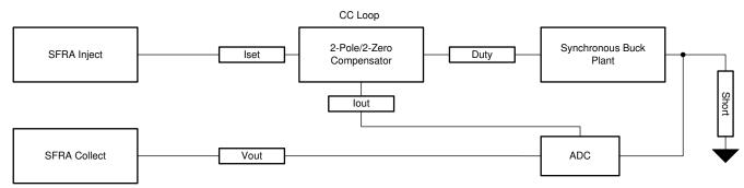
Figure 3-9. SFRA Setup Open-Loop CV Mode
