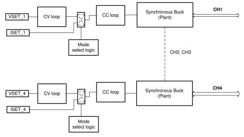
Figure 2-2. CCCV Feedback Controller
