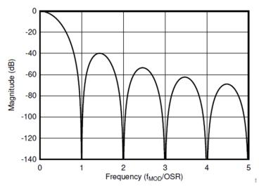
Figure 2-4. Sinc Digital Filter Response
