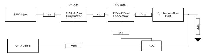
Figure 3-10. SFRA Setup Closed-Loop CV Mode
