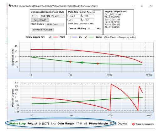
Figure 3-6. Tuning CC Loop Using Compensation Designer
