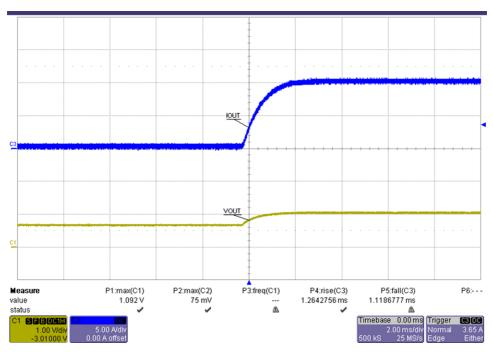
Figure 3-16. Output Current Transient Response
