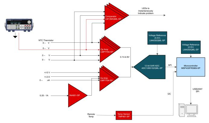
Figure 3-2. Voltage Monitor Test Setup
