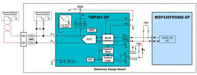
Figure 2-6. TMP461-SP - Local and Remote Temperature Sensing
