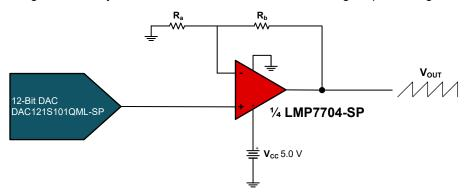
Figure 2-8. Adjustable Voltage Source
