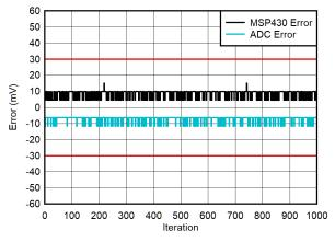
Figure 3-6. Noise Floor (20-V Range, 0-V Input)
