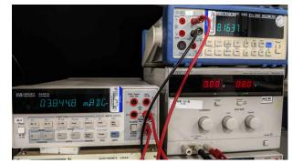
Figure 3-18. Constant Current Output Test Setup (8 V Applied)
