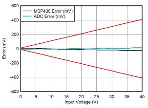
Figure 3-11. Linearity Plot (40-V Range)
