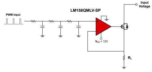
Figure 2-9. Fixed Output Current Source
