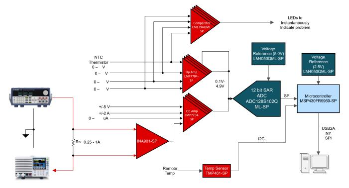
Figure 3-3. Current Monitor Test Setup
