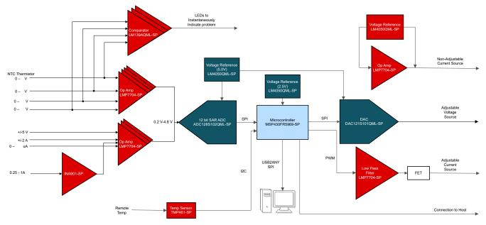
Figure 2-1. System Block Diagram (External ADC Configuration)
