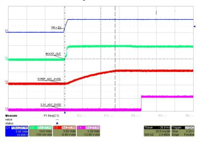
Figure 2-12. ADC128S102-SP Start-up Power Sequence
