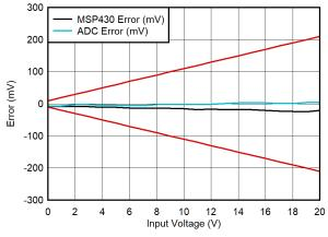
Figure 3-10. Linearity Plot (20-V Range)
