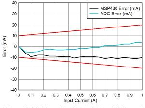
Figure 3-14. Linearity Plot (0.25- to 1-A Range)
