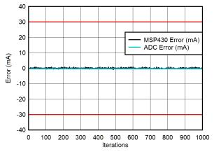
Figure 3-12. Noise Floor (0.25- to 1-A Range, 0 A, 5-V Input)
