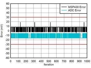
Figure 3-7. Noise Floor (40-V Range, 0-V Input)
