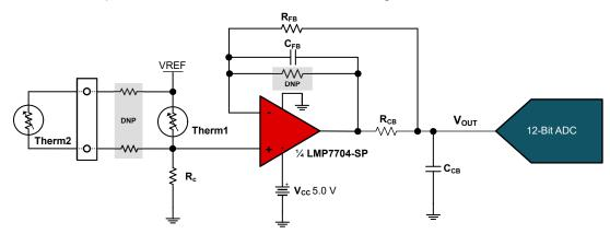
Figure 2-7. Thermistor Temperature Sensing
