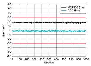
Figure 3-13. Noise Floor (±2-A Range, –2 A, 1-V Input)
