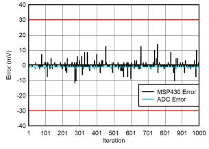
Figure 3-4. Noise Floor (5-V Range, 0-V Input)
