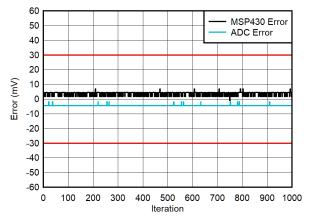
Figure 3-5. Noise Floor (±5-V Range, 0-V Input)
