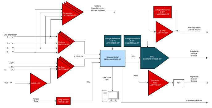
Figure 2-3. Voltage Monitoring - Internal ADC Configuration
