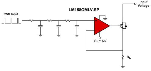
Figure 2-10. Adjustable Current Source Circuit
