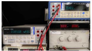
Figure 3-17. Constant Current Output Test Setup (7.5 V Applied)
