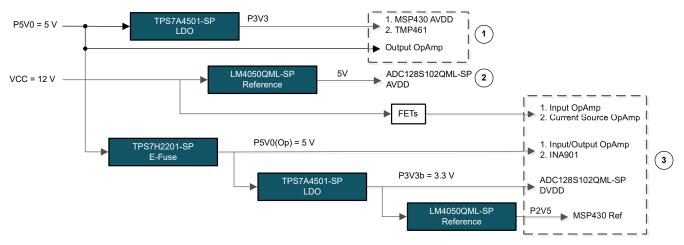
Figure 2-11. Power Tree and Sequencing
