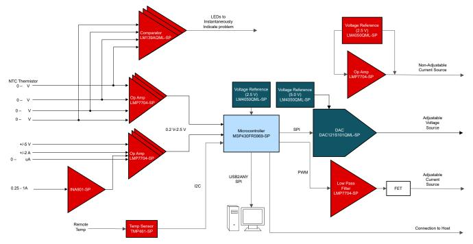
Figure 2-2. System Block Diagram (Internal ADC Configuration)
