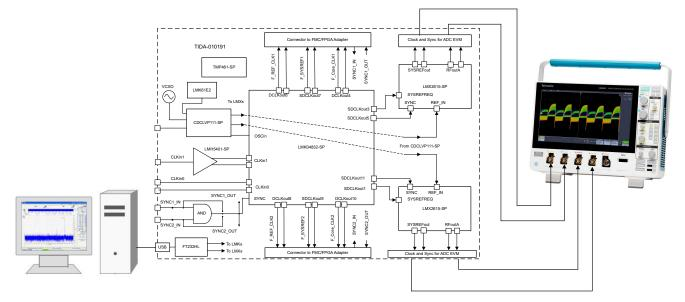
Figure 4-2. Test Setup for Multichannel Clock Skew Measurement
