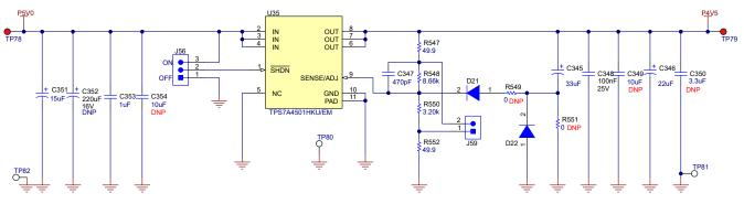
Figure 2-19. 0.75-A LDO for 4.5-V Supply With TPS7A4501
