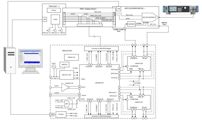
Figure 4-3. Test Setup for SNR Measurement
