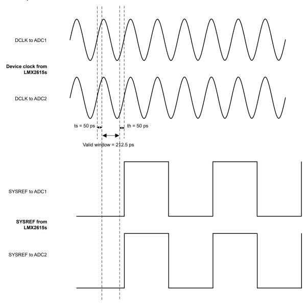
Figure 2-6. Clock and SYSREF Alignment
