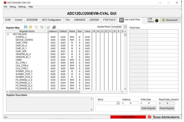
Figure 3-6. ADC12DJ3200 EVM Programming
