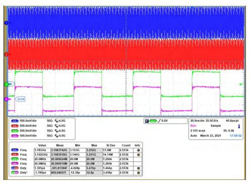
Figure 4-8. Scope-Shot Multichannel Clock Phase Alignment
