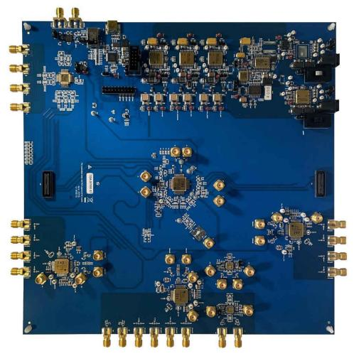
Figure 3-1. TIDA-010191 Clocking Board
