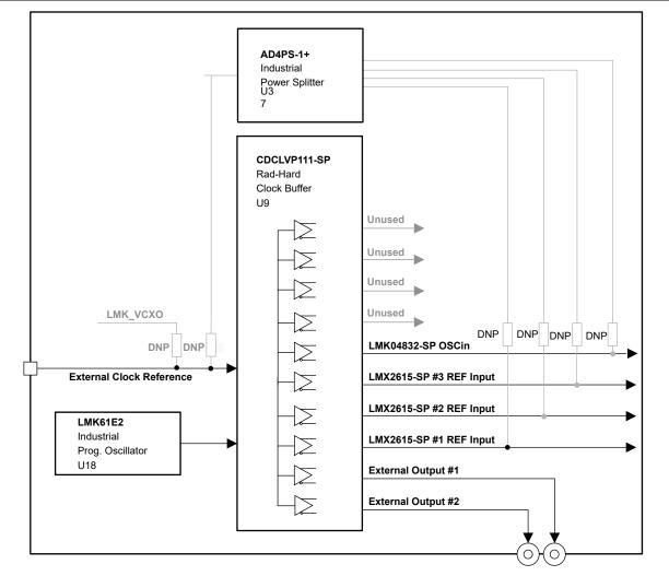
Figure 2-5. Passive Clock Distribution Using Power Splitter
