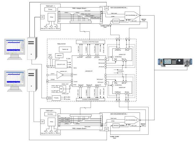
Figure 4-4. Test Setup for Channel-to-Channel Skew Measurement
