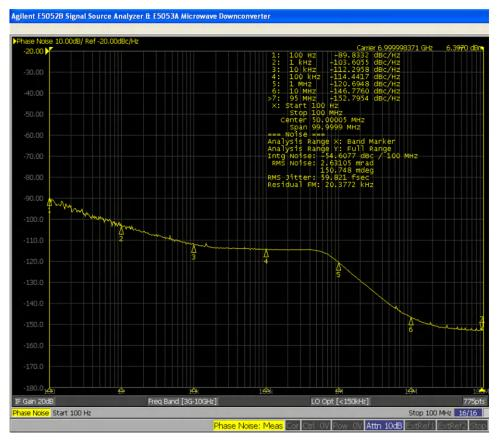
Figure 4-5. Phase Noise at 7-GHz Carrier Frequency
