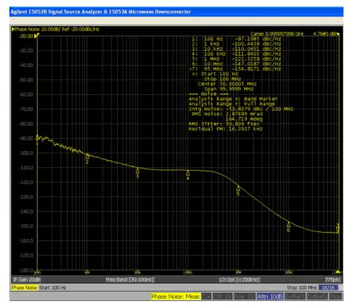
Figure 4-6. Phase Noise at 9-GHz Carrier Frequency
