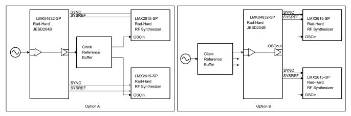
Figure 2-4. Clock Distribution Options A and B
