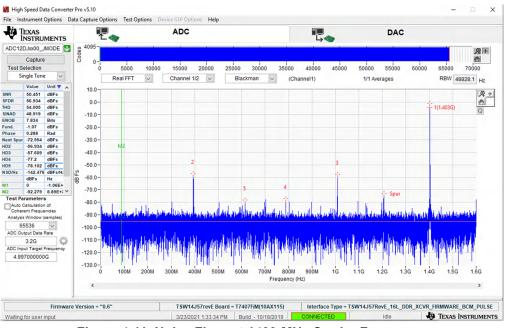
Figure 4-11. Noise Floor at 1403-MHz Carrier Frequency
