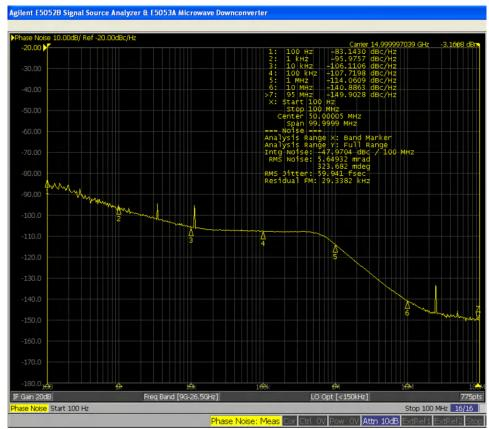
Figure 4-7. Phase Noise at 15-GHz Carrier Frequency
