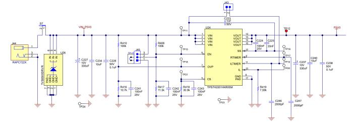
Figure 2-14. One Branch of Redundant eFuse
