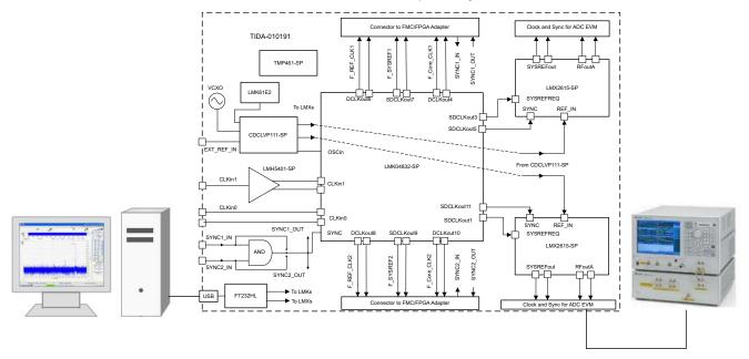
Figure 4-1. Test Setup for Phase Noise Measurement
