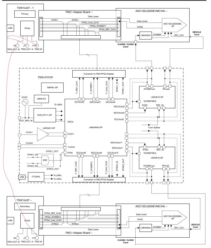
Figure 2-1. Measurement System Setup
