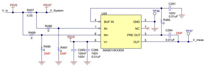
Figure 2-20. Power Supply Current Sensing
