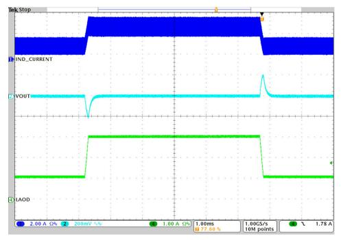
Figure 3-4. Load Transient 1-A to 3-A with 12-Vin
