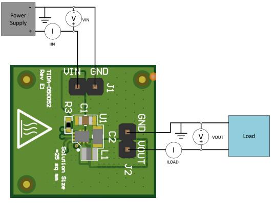
Figure 3-1. Test Setup
