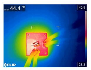
Figure 3-11. Thermal Image at Room Temperature with 12-Vin, 1.2-Vo, 1-A.
