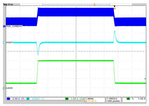
Figure 3-3. Load Transient 500-mA to 3-A with 12-Vin
