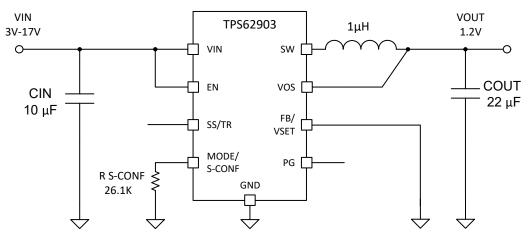
Figure 2-1. TIDA-050052 Block Diagram
