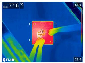
Figure 3-9. Thermal Image at Room Temperature with 12-Vin, 1.2-Vo, 3-A
