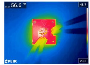
Figure 3-10. Thermal Image at Room Temperature with 12-Vin, 1.2-Vo, 2-A
