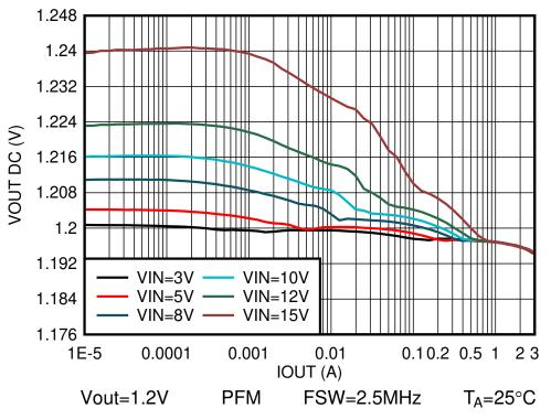
Figure 3-12. Output Voltage vs. Output Current at Room Temperature
