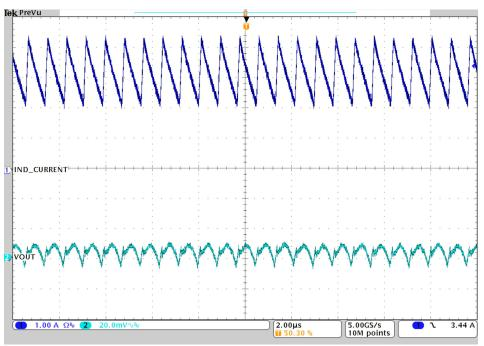
Figure 3-7. Vout ripple at 3-A
