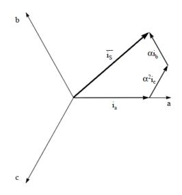
Figure 2-4. Stator Current Space Vector and its Component in (a,b,c) Frame
