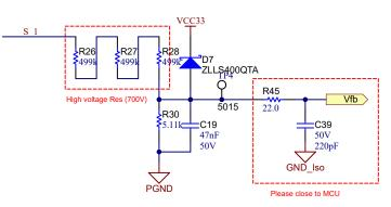
Figure 2-20. Motor Voltage Sensing Circuit
