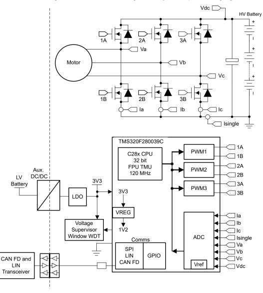
Figure 2-1. TIDM-02012 eCompressor Block Diagram
