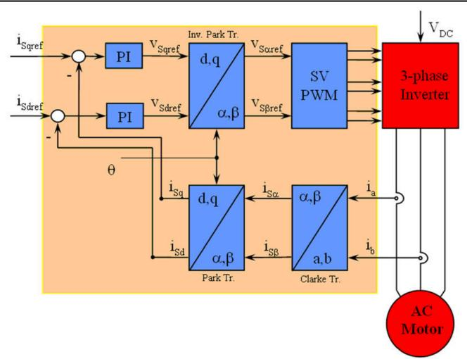
Figure 2-7. Basic Scheme of FOC for AC Motor
