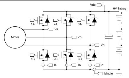
Figure 3-1. Hardware Board Block Diagram of TIDM-02012
