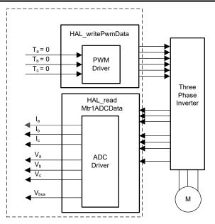
Figure 3-7. Build Level 1 Software Block Diagram
