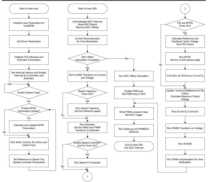
Figure 2-14. Flowchart for an InstaSPIN-FOC Project with FW and MTPA
