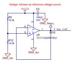
Figure 2-17. 1.65-V Reference from 3.3-V Input Circuit
