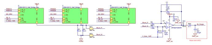
Figure 2-19. Motor Current Sensing Circuit with Single-Shunt
