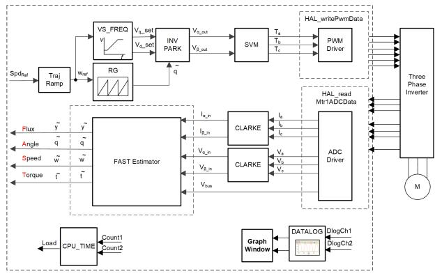
Figure 3-9. Build Level 2 Software Block Diagram
