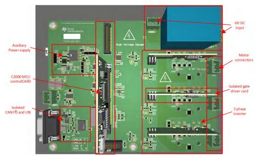
Figure 3-2. The Layout of eCompressor Reference Design Board
