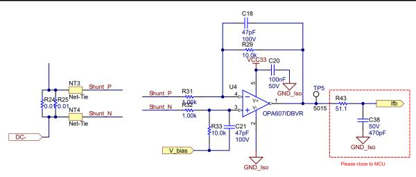
Figure 2-18. Motor Current Sensing Circuit with Three-Shunt
